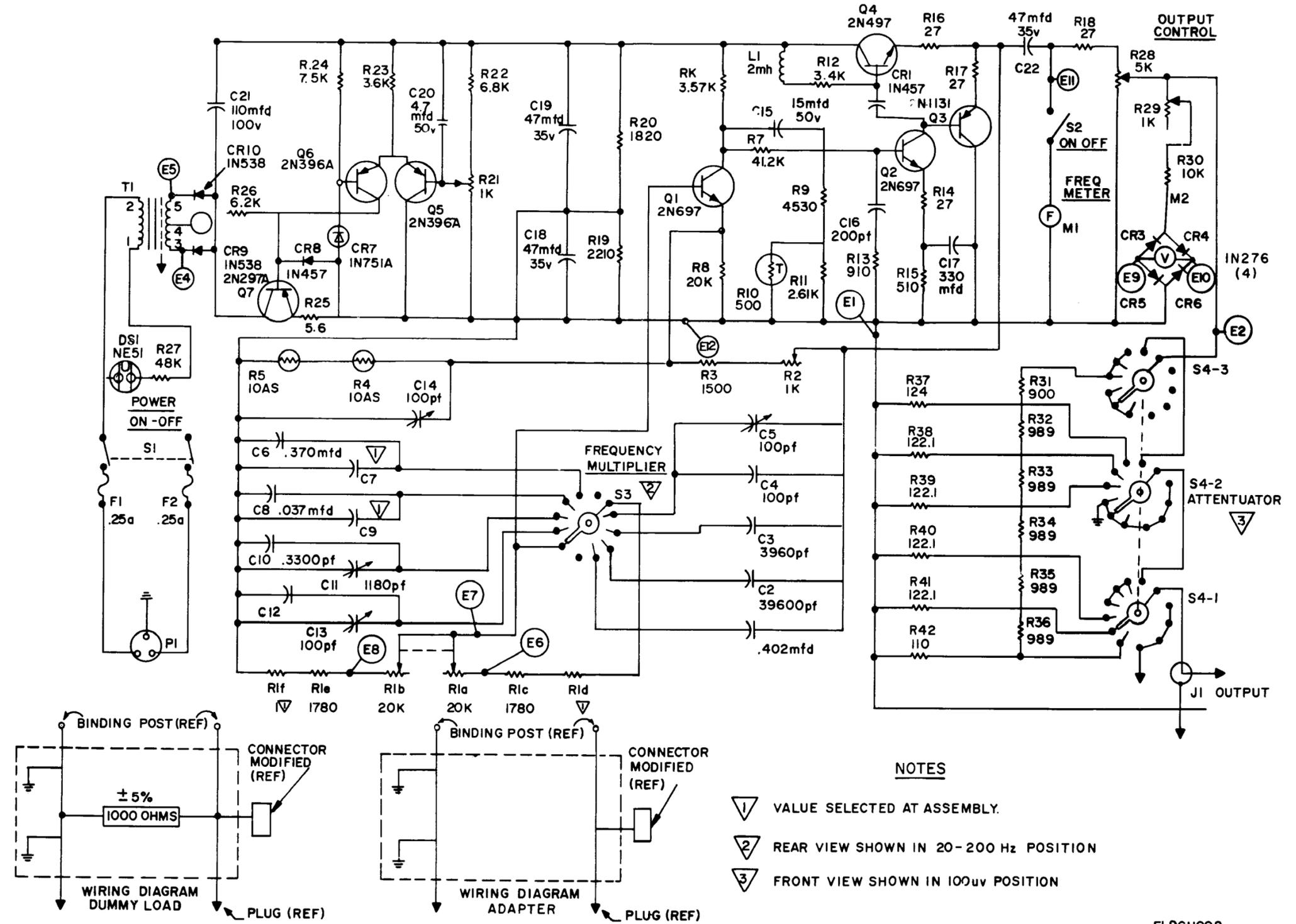
FO-3 AN/URM-127 Signal Generator Schematic Diagram.
