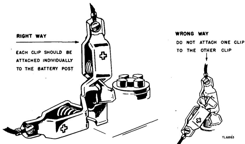
Figure 8. Battery terminal connections.
