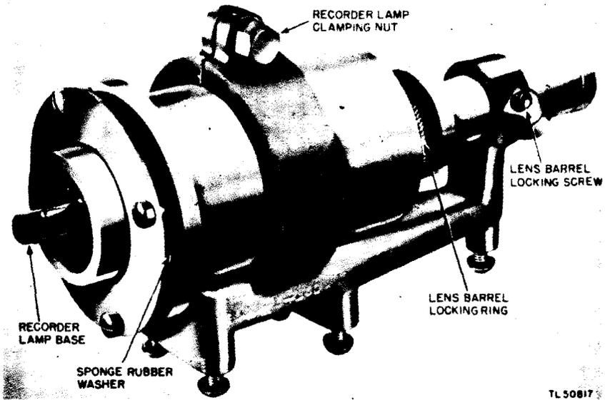
Figure 15. Recorder lamp assembly of Facsimile Transceiver FX-1-A.
