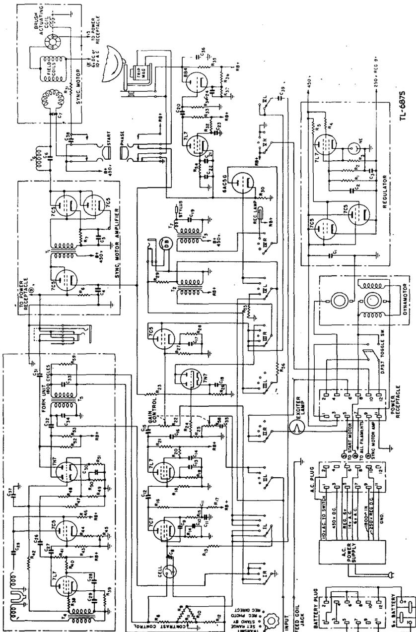
Figure 42. Schematic circuit diagram of Facsimile Transceiver FX-1.
