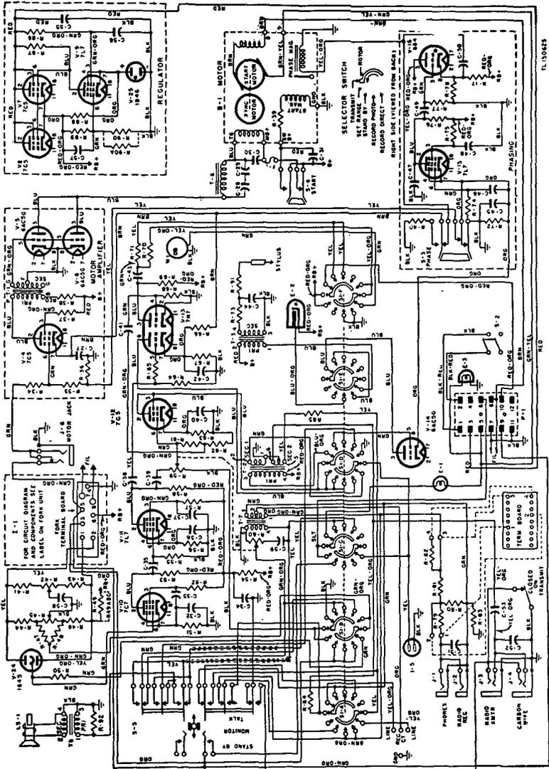
Figure 44. Schematic circuit diagram of Facsimile Set AN/TXC-1A.
