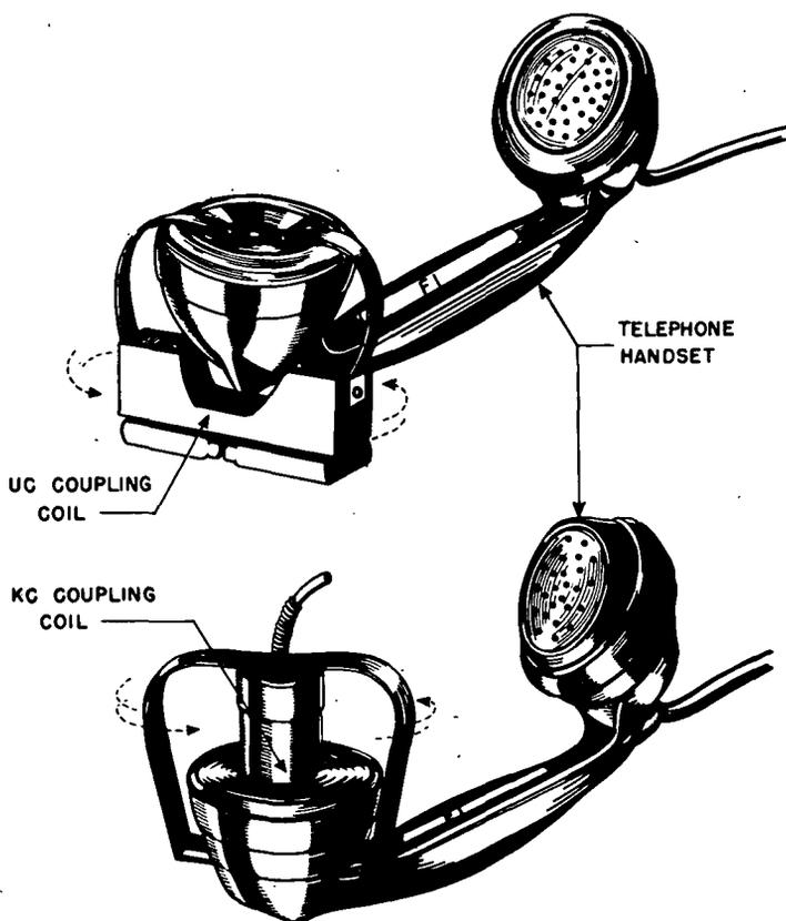
TURN COUPLING UNITS TO OBTAIN MAXIMUM PICKUP AS INDICATED BY THE LOUDEST SIGNAL FROM THE EAR-PIECE.
