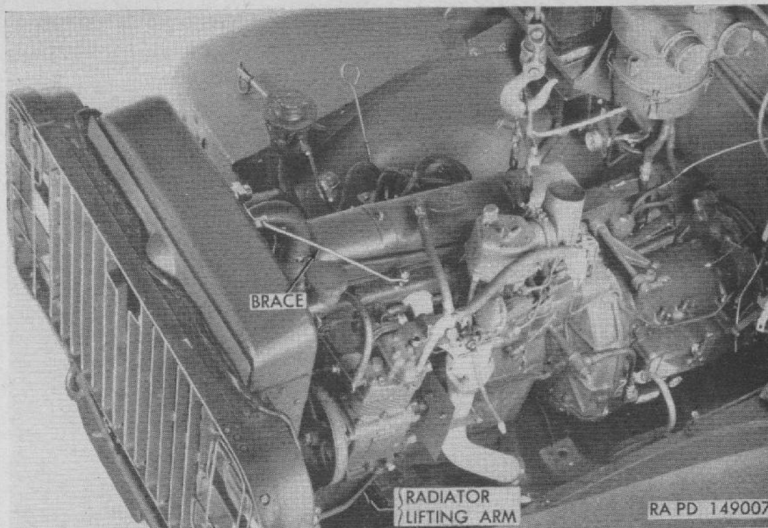
Figure 41. Removing power plant showing radiator brace.
