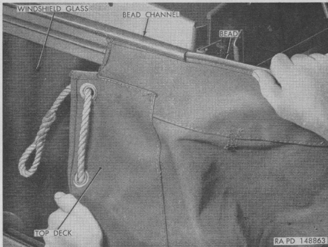
Figure 162. Removing top deck from windshield channel.
