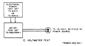
Figure 4. Connections for final tests.
