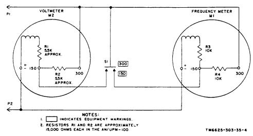
Figure 1. Schematic diagram.
