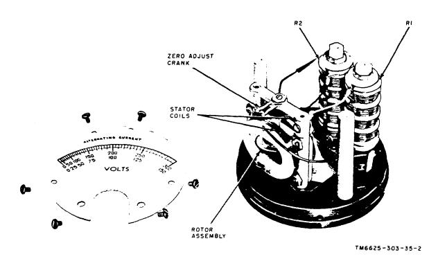
Figure 2. Voltmeter M2, interior view.
