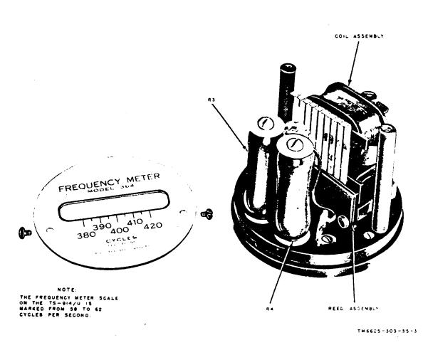
Figure 3. Frequency meter M1, interior view (TS-934/U).
