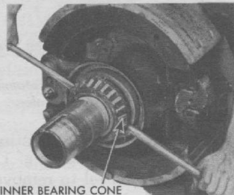
Removing inner bearing cone
