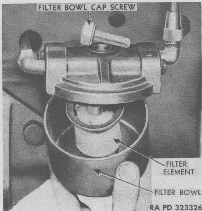
Figure 48 — Removing Fuel Filter Bowl
