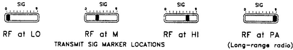
**SIG** (signal) display. Shows approximate signal strength. Marker lights further right for stronger signals. RF switch setting determines the amount of signal strength while transmitting.
