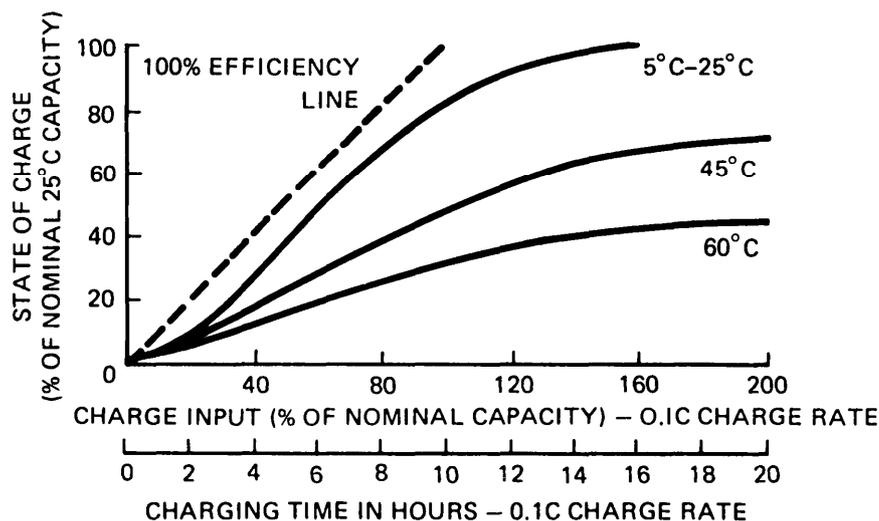
At low temperatures, the batteries cannot fully discharge even if they were fully charged at room temperature. At high temperatures, this same effect takes place to a lesser degree, in addition to the problem of charge acceptance previously mentioned.
