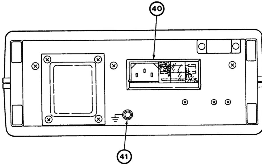
Figure 4-2. Operator’s Controls, Indicators, and Connectors, rear view.
