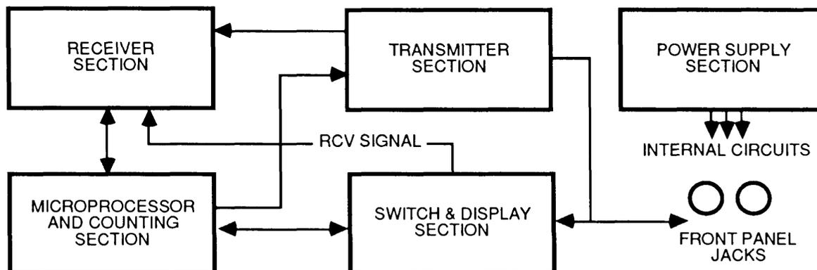
Figure 3-1. AN/USM-485 Simplified Block Diagram.
