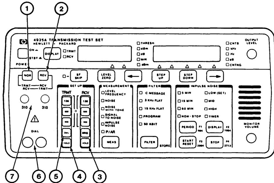
1. Connect circuit to left TRMT/RCV jack (7).
