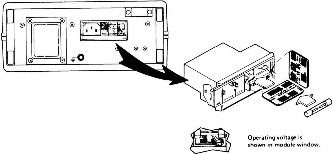
6. Rotate FUSE-PULL back into normal position and reinsert fuse. Use table below to select correct fuse value.
