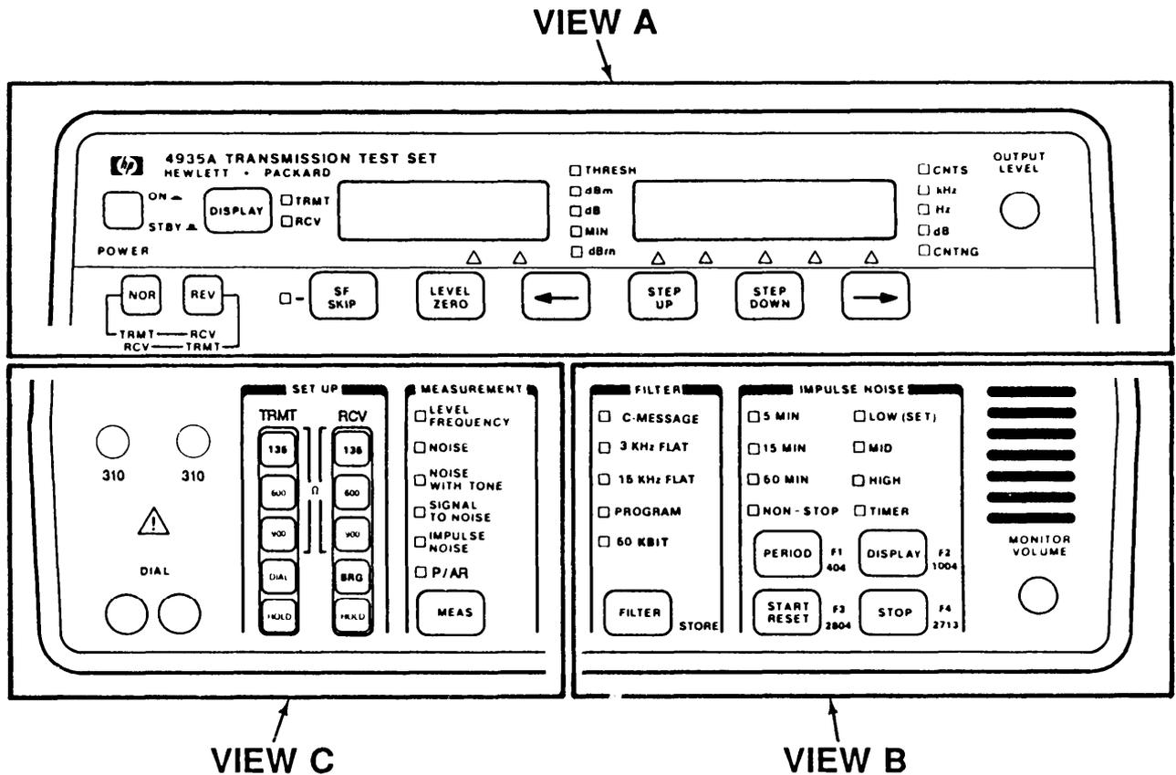
Figure 4-1. Operator's Controls, Indicators, and Connectors, front view.
