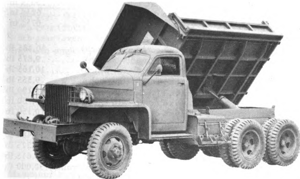
Figure 9—148-inch W.B. Side Dump Model Truck US 6— Body Raised
