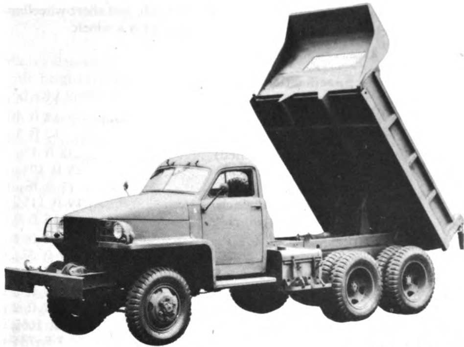
Figure 8—148-inch W.B. End Dump Model Truck US 6— Body Raised
