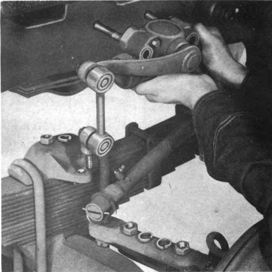
Figure 195—Removing Shock Absorber
