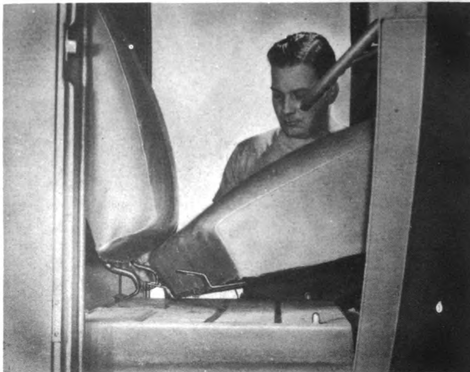
Figure 200—Removing Seat Cushion
