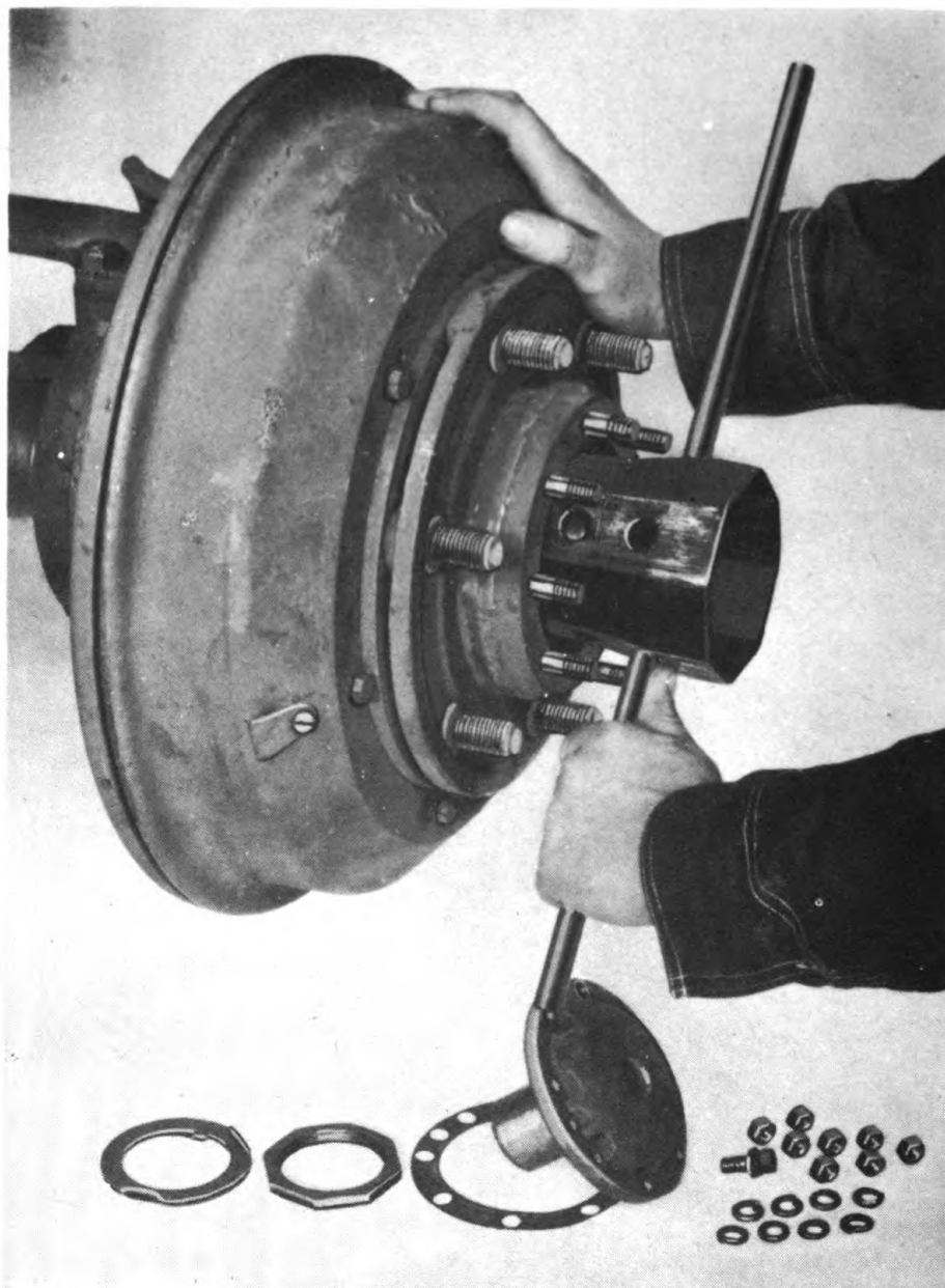
Figure 174—Adjusting Front Wheel Bearings (6 x 6)
