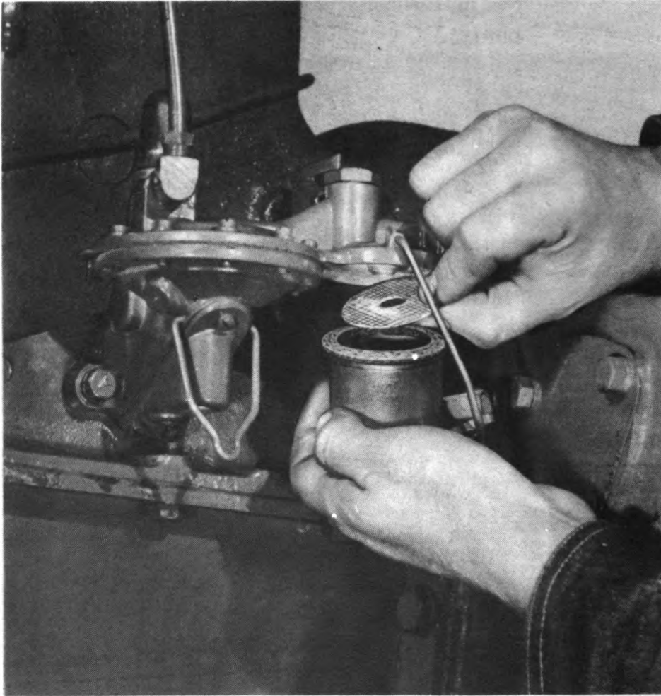
Figure 77—Removing Fuel Pump Screen
