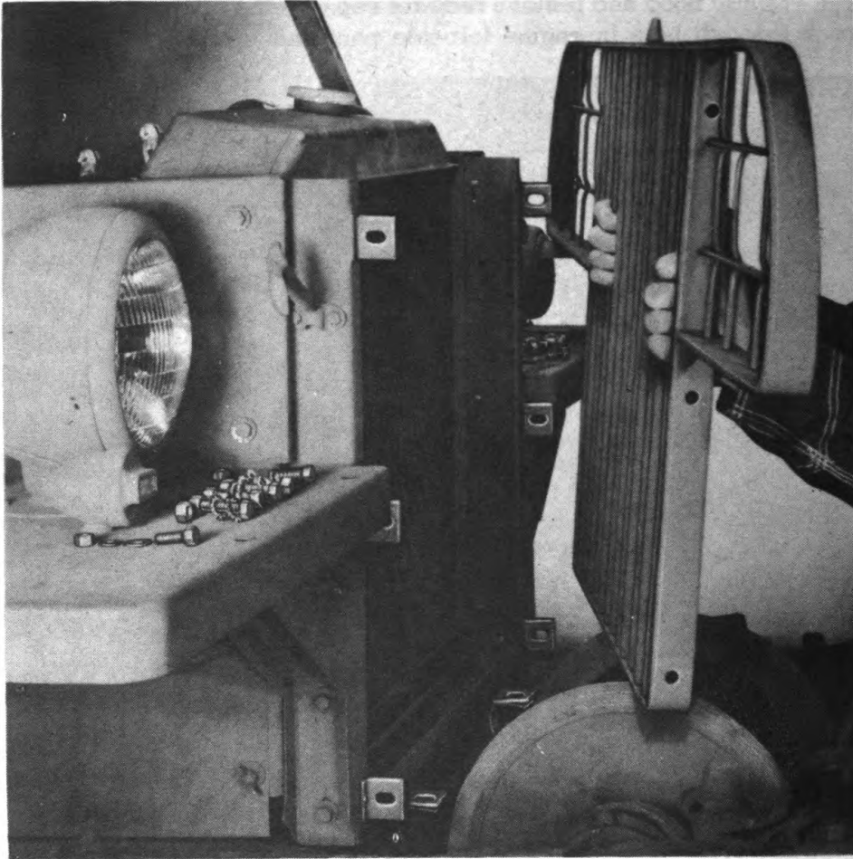
Figure 88—Removing Radiator Guard
