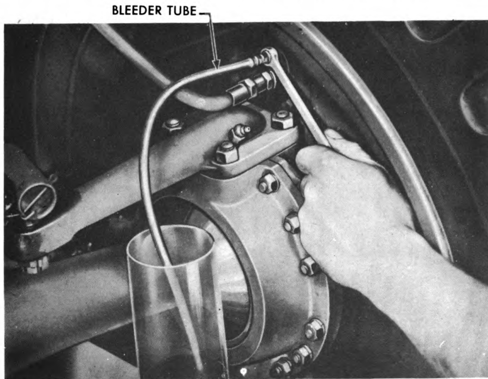
Figure 144—Bleeding Wheel Cylinder RA PD 319216
