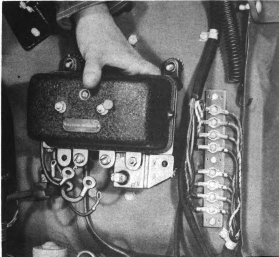
Figure 99—Removing Generator Regulator
