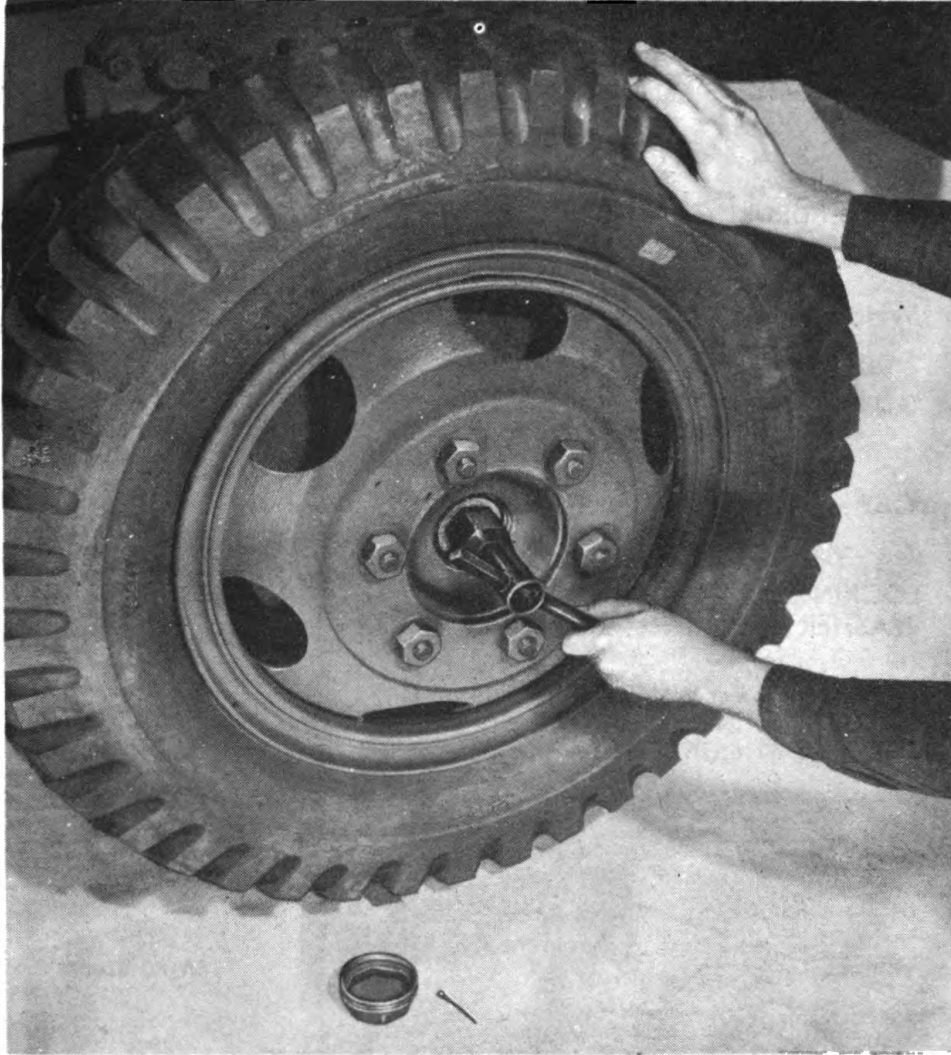
Figure 182—Adjusting Front Wheel Bearings (6 x 4)
