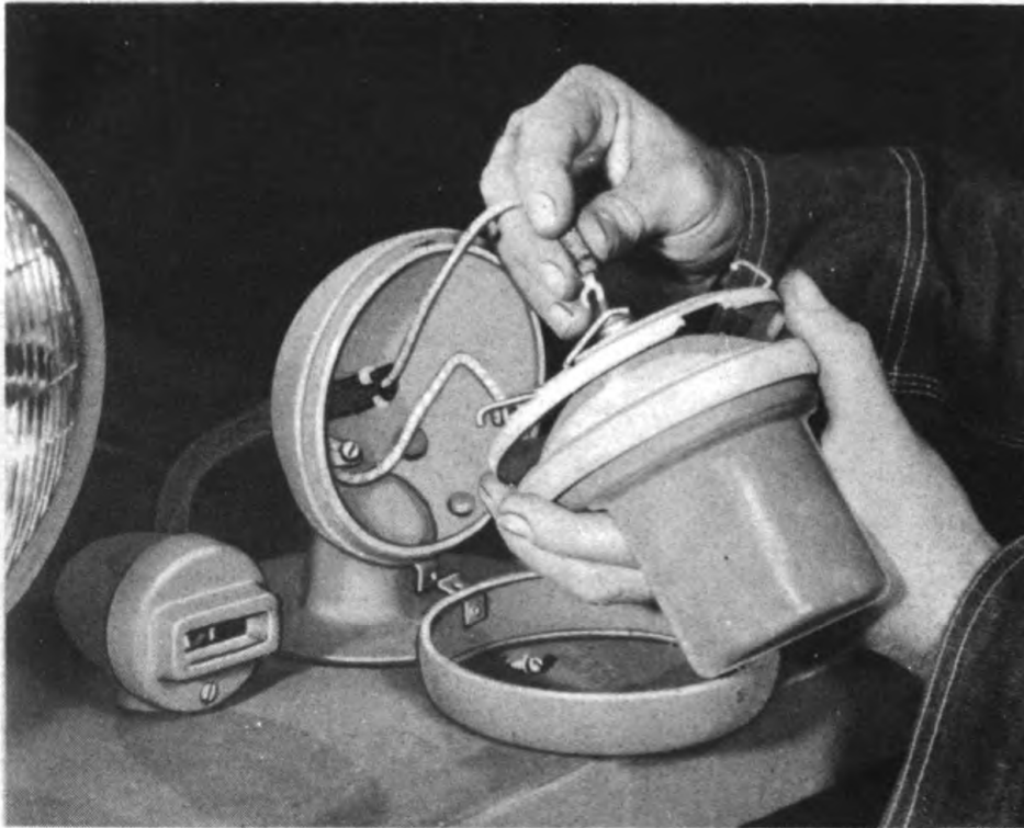
Figure 212—Replacing Blackout Driving Light Lamp Unit
