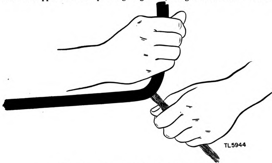
Figure 32. Method of separating rubber jacket from conductors.
