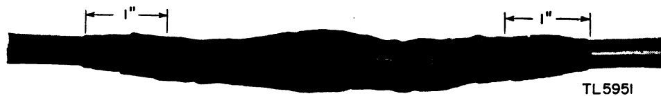
Figure 39. Friction tape applied to splice.
