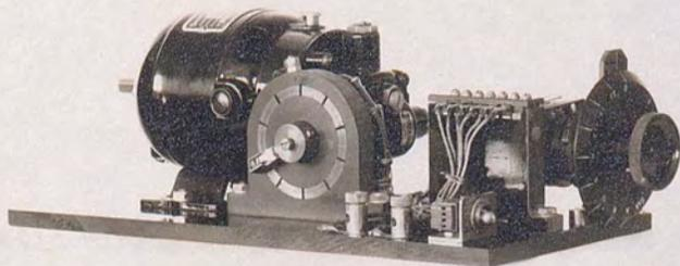
Fig. 2 - Distributor and Selector for Keying Signal Equipment SE-7-T1
