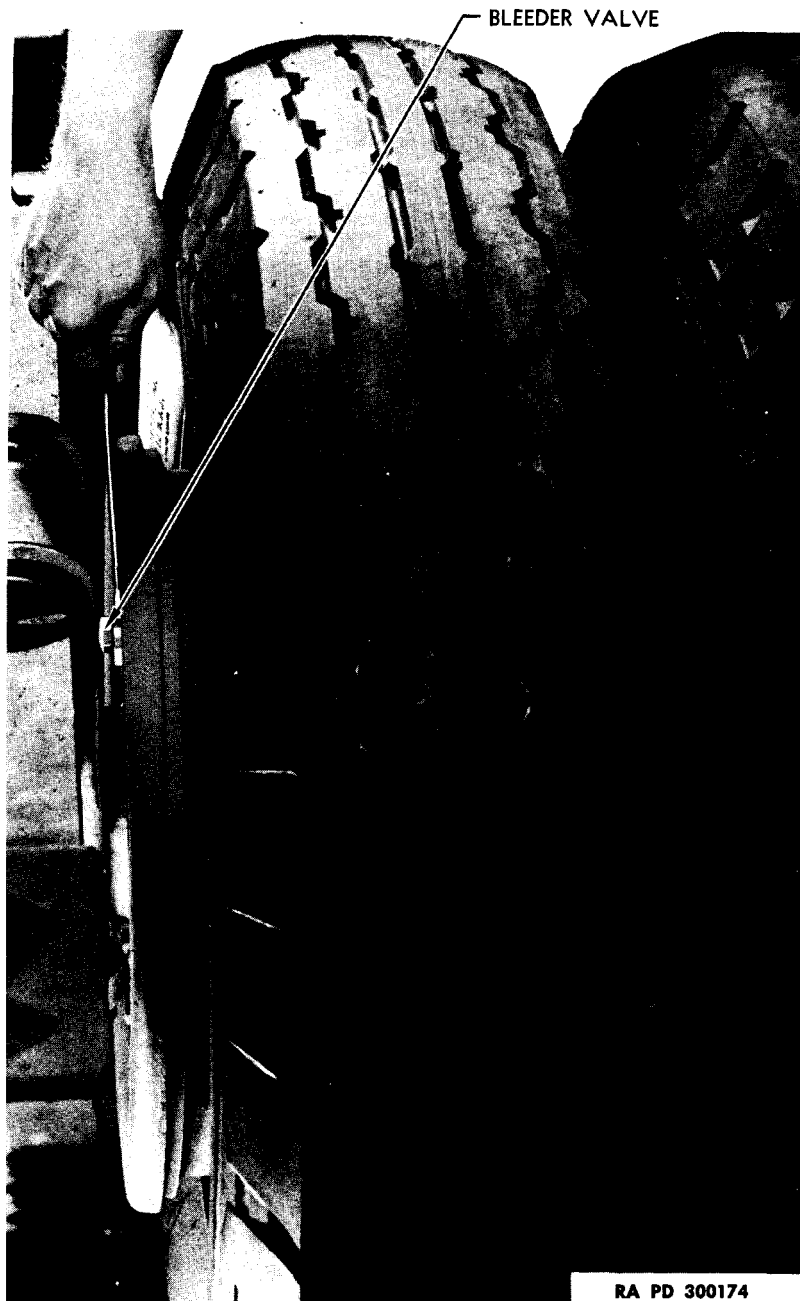
Figure 84—Bleeding Rear Brake
