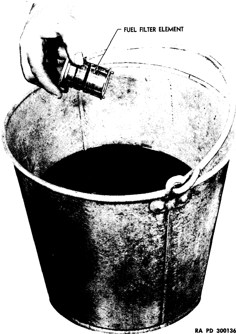
Figure 42—Cleaning Fuel Filter Element
