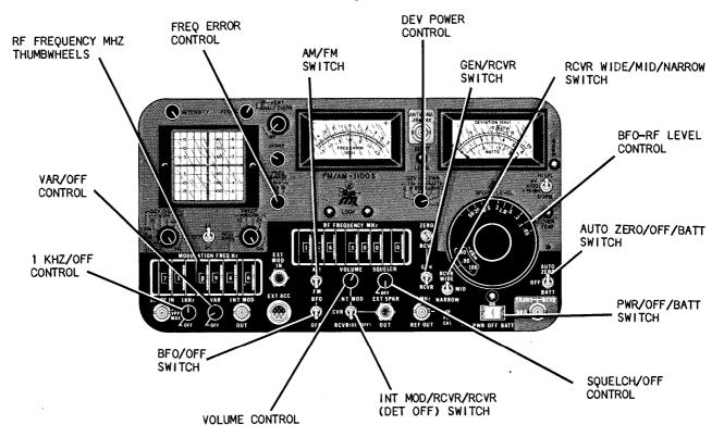
Figure 2-16 FM/AM-1100S Initial Adjustments and Control Settings for Master Oscillator Calibration Using Received Time Standard Signal (WWV)
