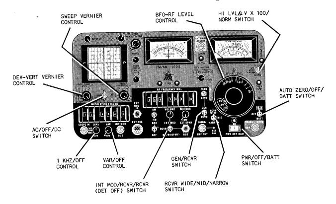
Figure 2-8 FM/AM-1000S Initial Adjustments and Control Settings for Generating AM RF Signals
