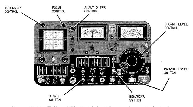
Figure 2-12 FM/AM-1100S Initial Adjustments and Control Settings for Spectrum Analyzer Operation
