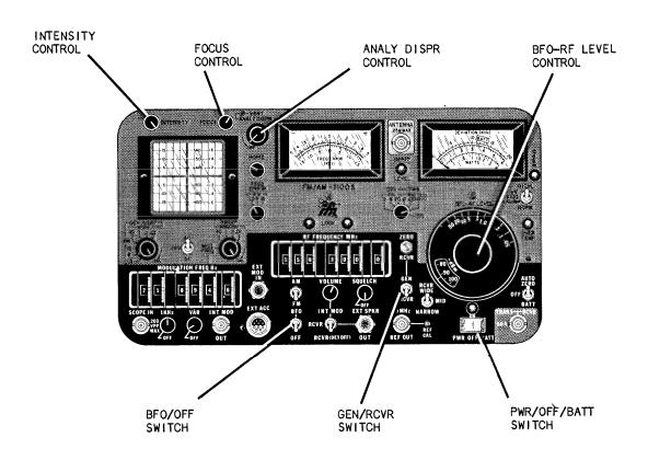
Figure 2-13 FM/AM-1100S Initial Adjustments and Control Settings for Spurious Signal Detection Using Spectrum Analyzer
