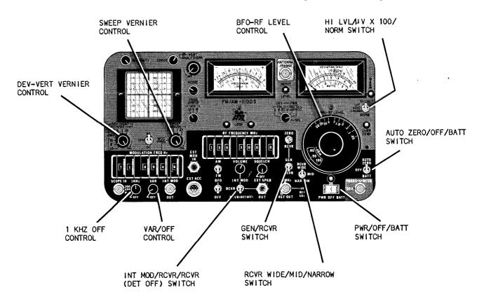
Figure 2-9 FM/AM-1100S Initial Adjustments and Control Settings for Generating FM RF Signals
