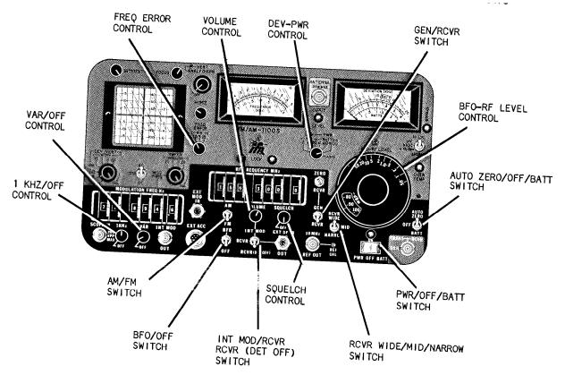
Figure 2-11 FM/AM-1100S Initial Adjustments and Control Settings for Receiver Operation
