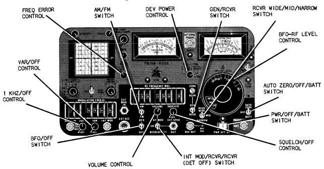
Figure 2-15 FM/AM-1100S Initial Adjustments and Control Settings for Measuring Transmitter Carrier Power
