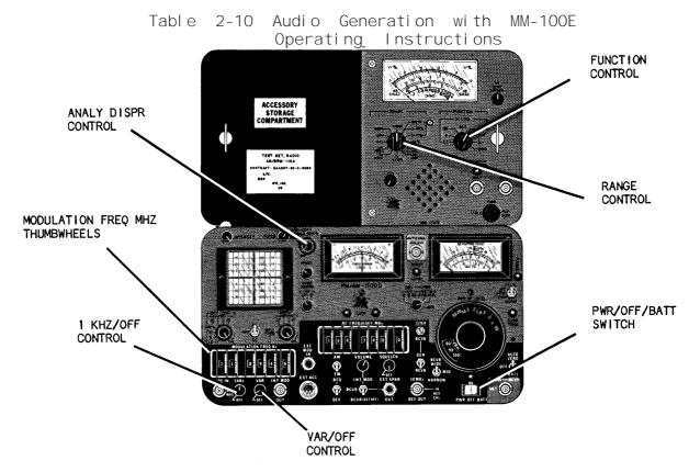
Figure 2-14 FM/AM-1100S and MM-100E Initial Adjustments and Control Settings for Generating Audio Signals
