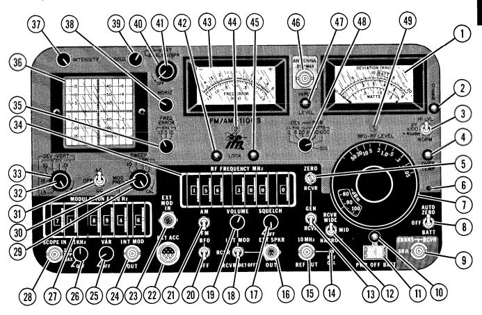
Figure 2-1 FM/AM-1100S Front Panel
