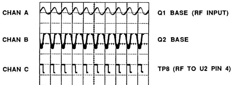
Figure SS8-2. RF Amplifier Waveforms (CHANGE 10)
