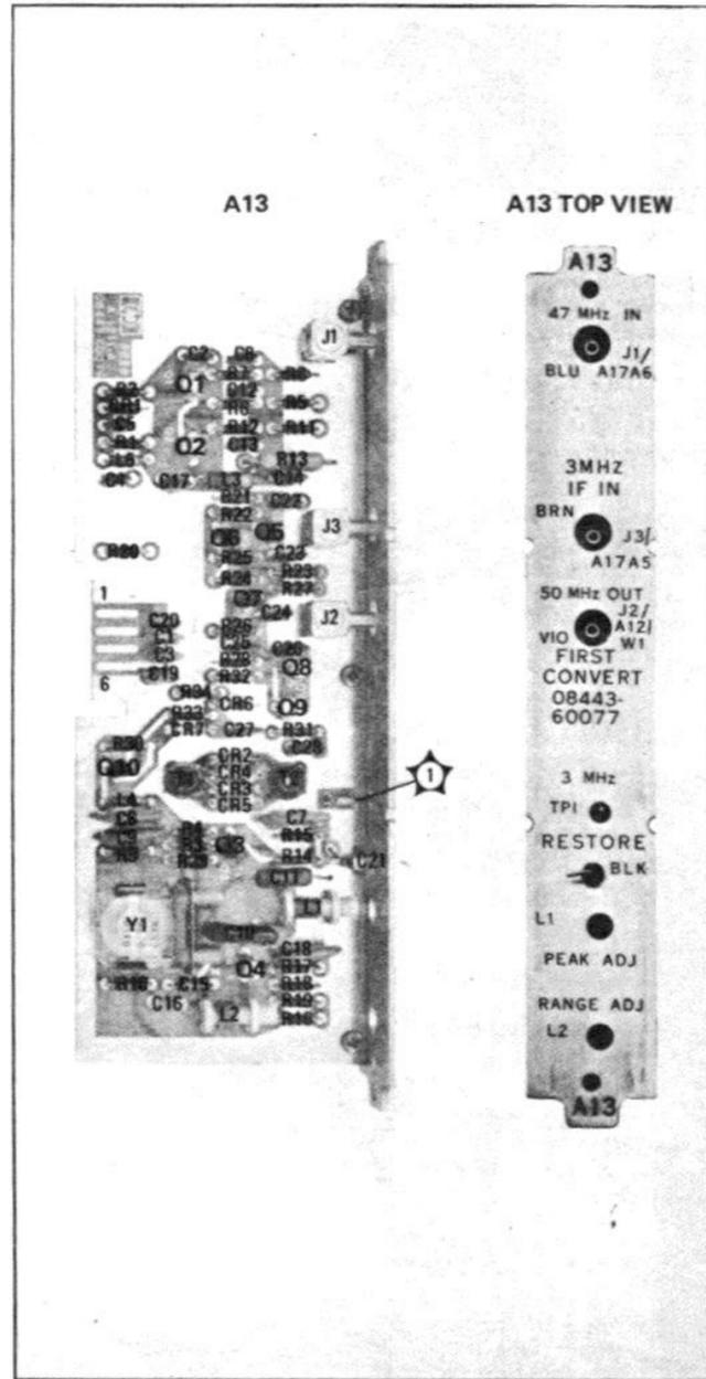
Figure 8-21. A13, First Converter, Cover and Components
