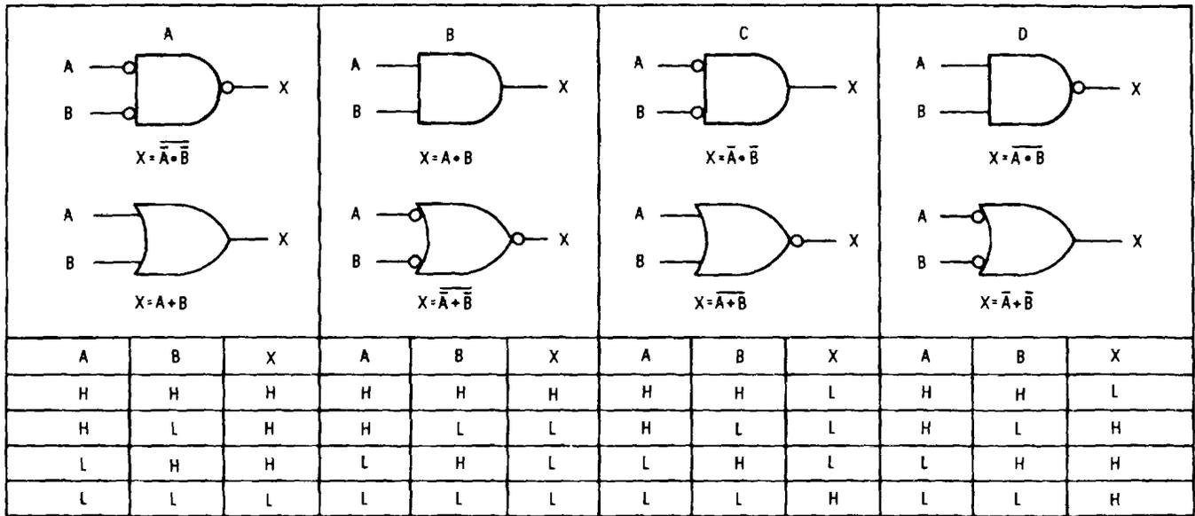
Figure 8-4. Logic Comparison Diagrams
