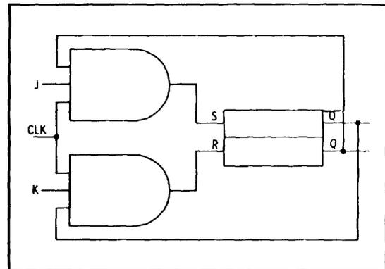
Figure 8-9. Clocked JK Flip-Flop
