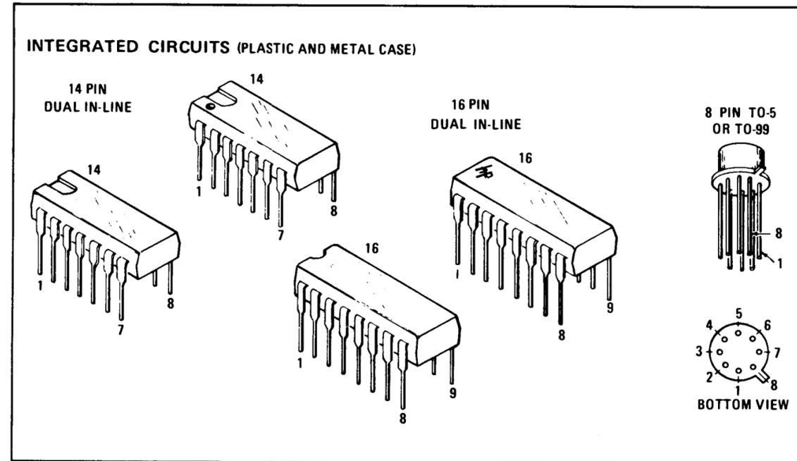
Figure 8-16. Integrated Circuit Packing
