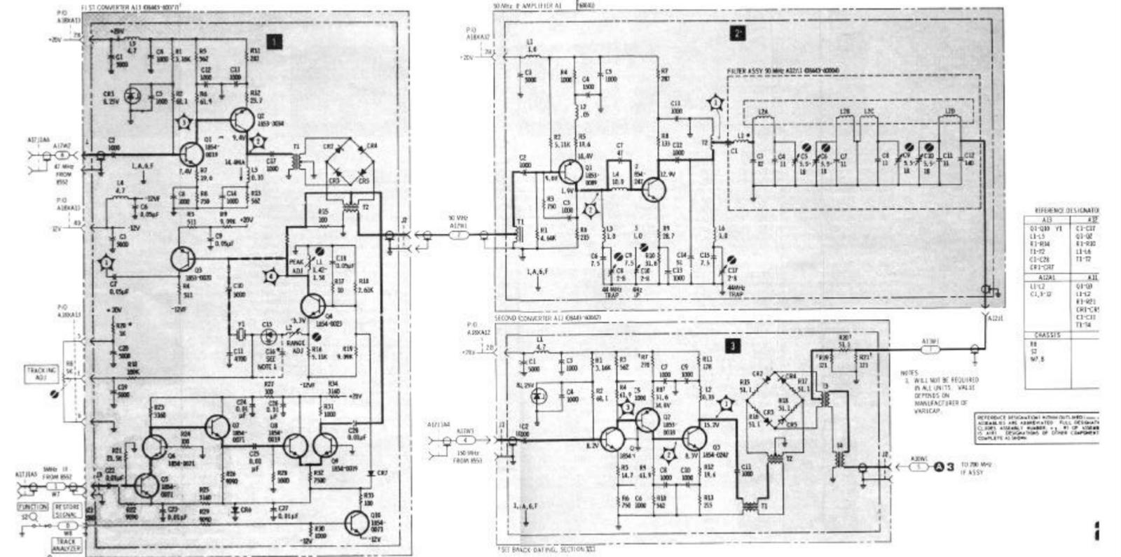
Figure 8-23. First and Second Converter and IF Amplifier, Schematic Diagram
