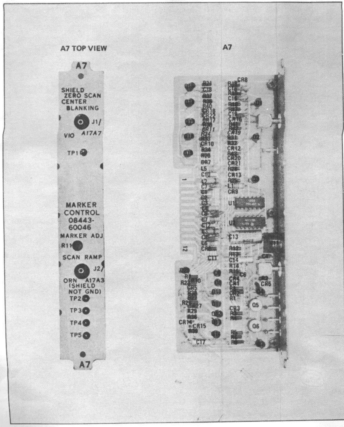
Figure 8-32. A7, Marker Control Assembly, Cover and Components
