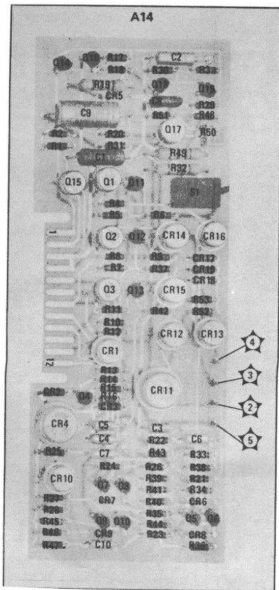
Figure 8-28. A14, Sense amplifier Assembly, Components
