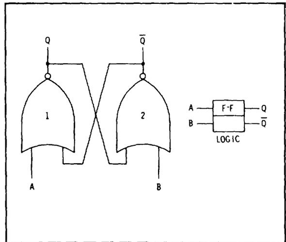
Figure 8-5. Basic NOR Gate Flip-Flop
