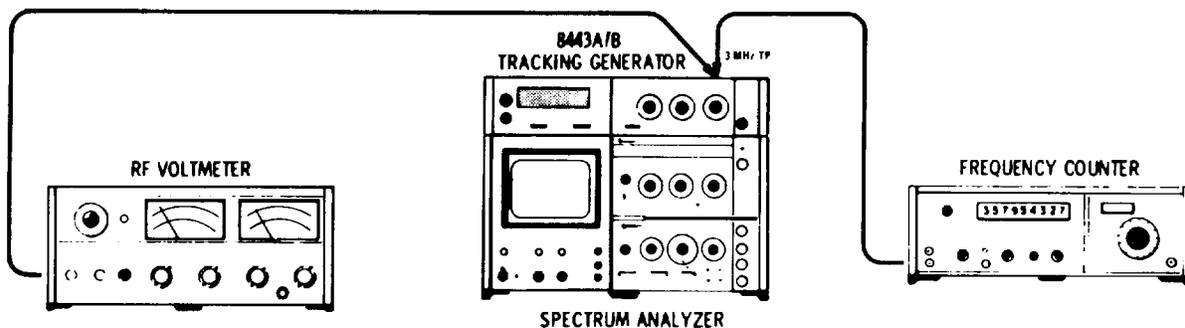
Figure 5-2. First Converter Test Setup
