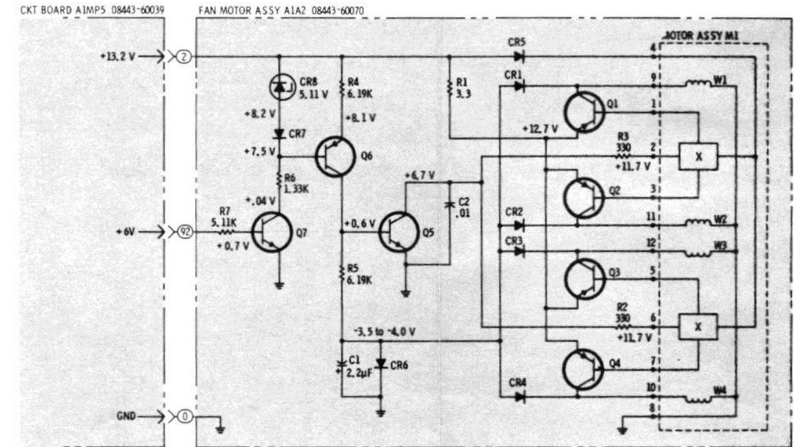
Figure 8-42. Fan Motor Credits, Schematic Diagram
