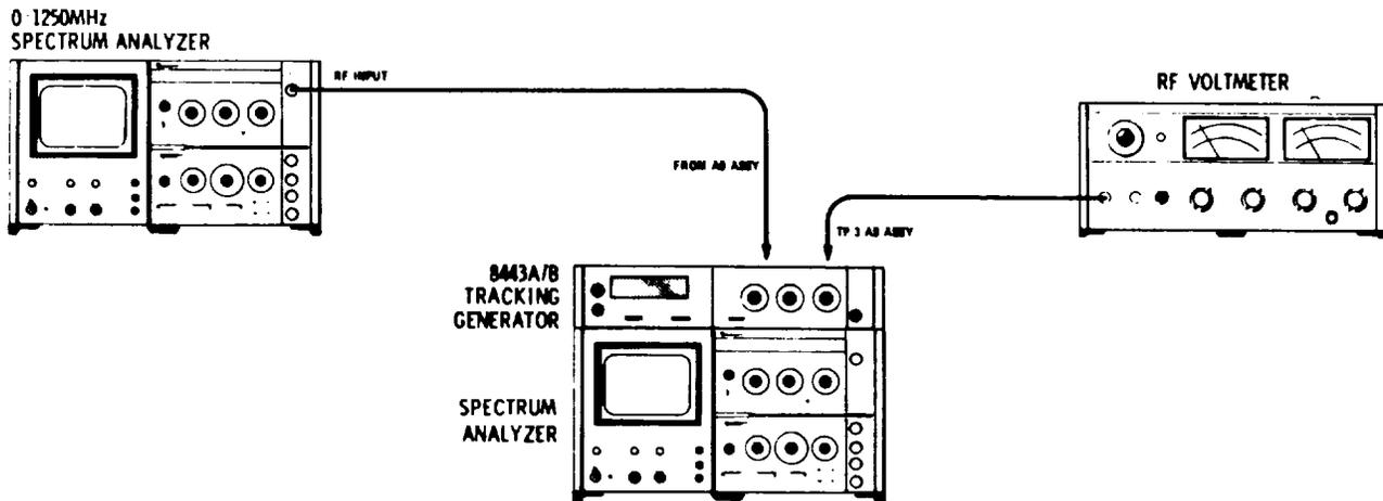
Figure 5-4. Third Converter Test Setup
