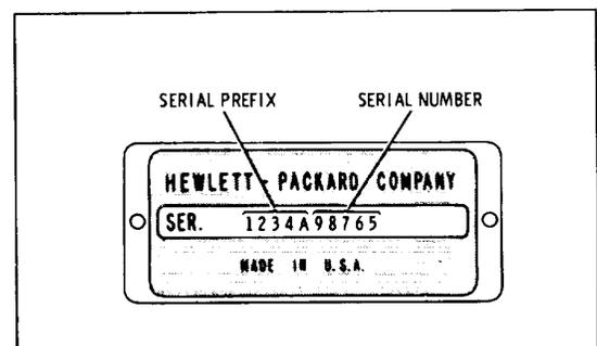
Figure 1-2. Instrument Identification
