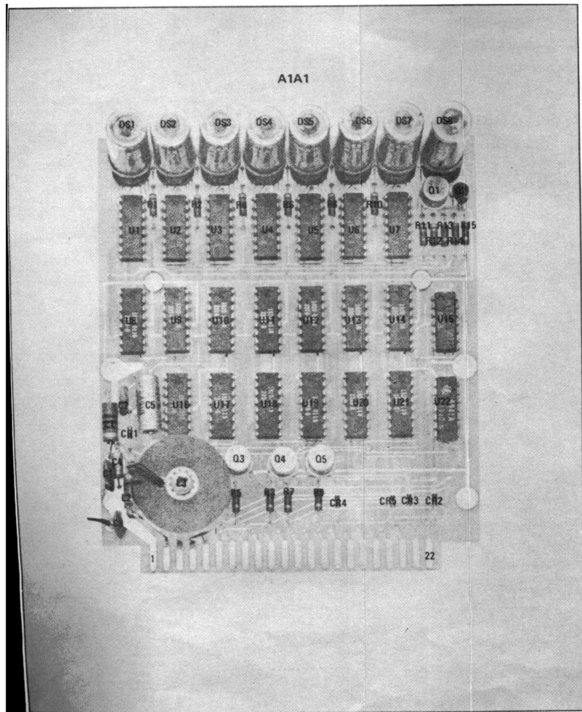
Figure 8-38. A1A1, Low frequency Counter Board Assembly, Components
