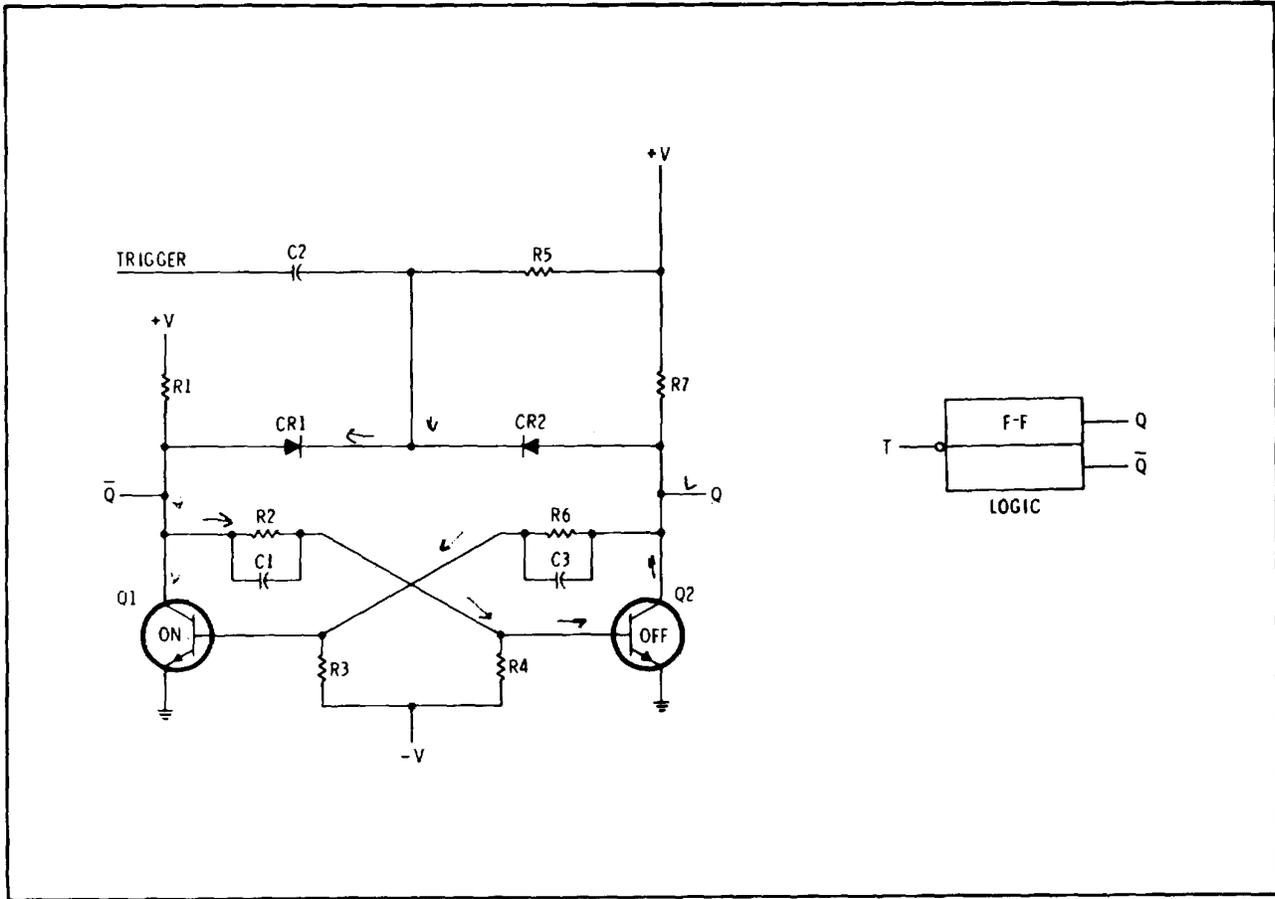
Figure 8-6. Triggered Flip-Flop
