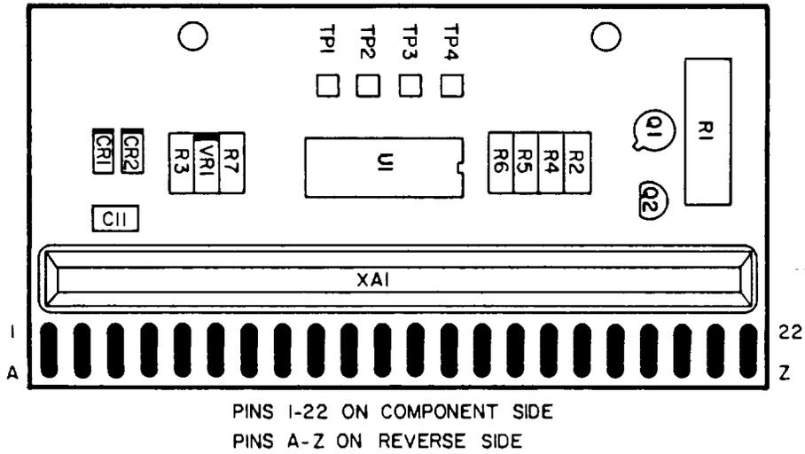
Figure 8-38C. A1A3, +6V Switched Board Assembly, Components (CHANGE 9)
