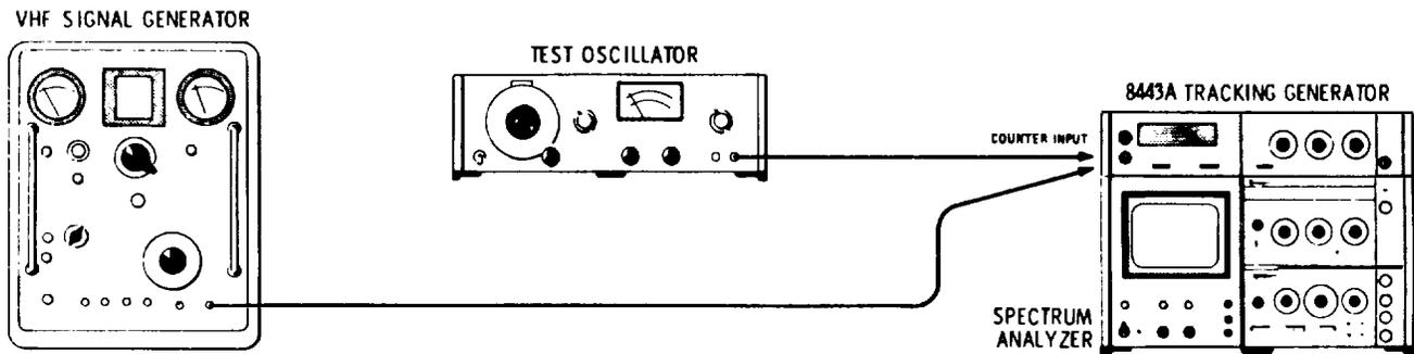
Figure 4-6. Counter Input Test Setup
