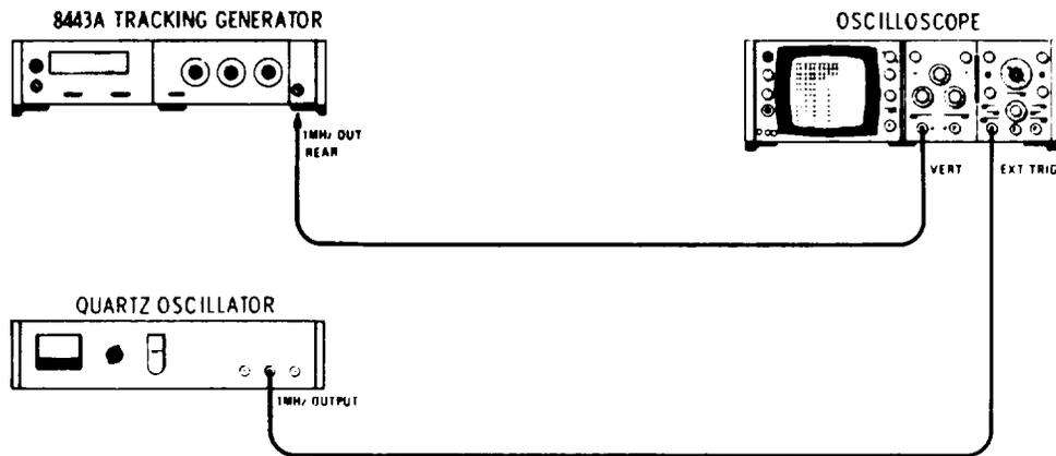
Figure 5-6. Reference Oscillator Test Setup
