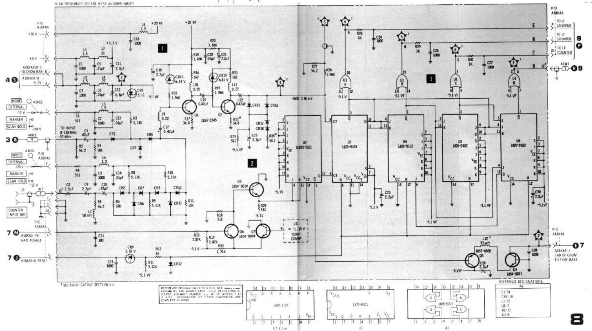
Figure 8-37. High Frequency Decade Assembly, Schematic Diagram
