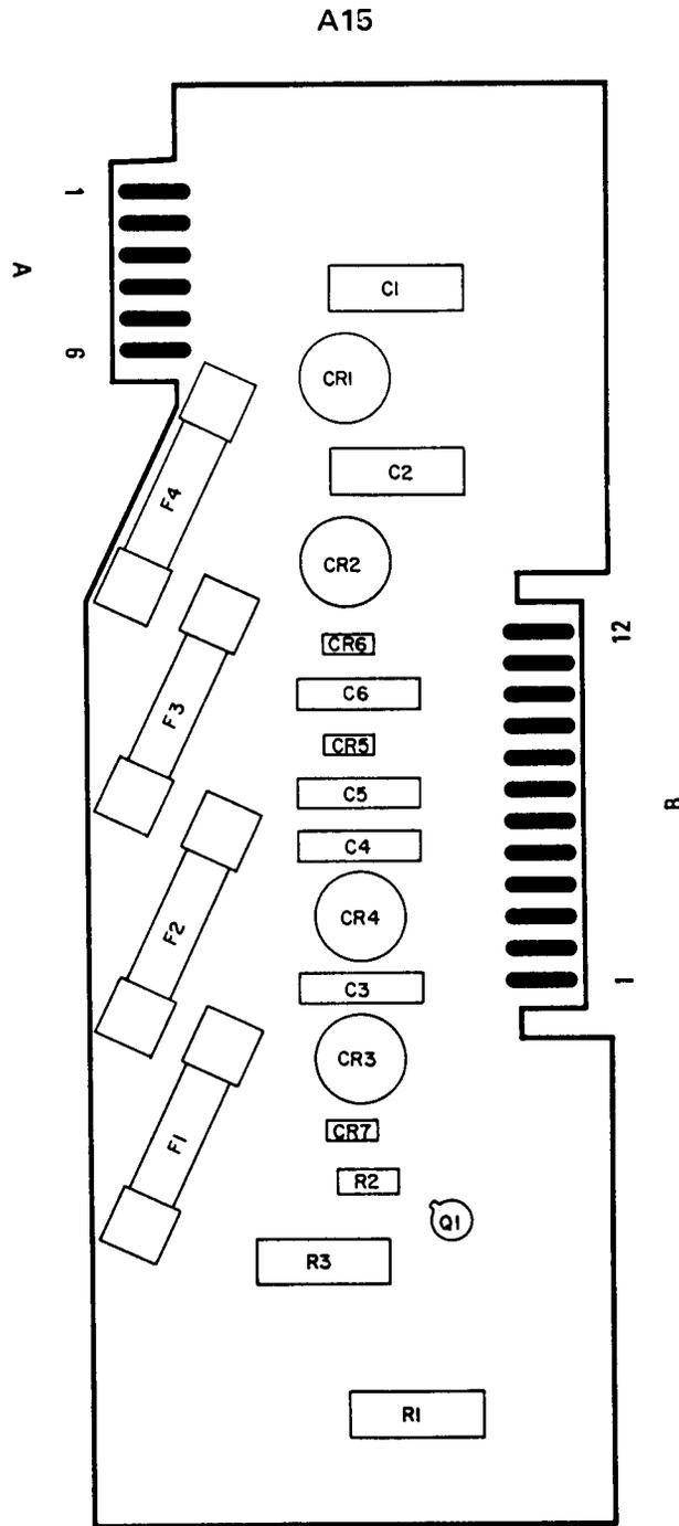
Figure 8-29. A15, Rectifier Assembly, Components (CHANGE 12)
