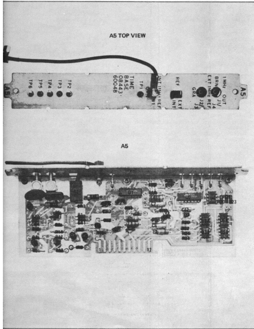
Figure 8-34. A5, Time Base Assembly, Cover and Components
