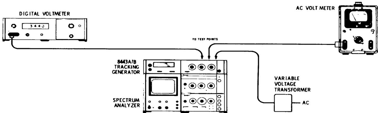
Figure 5-1. Power Supply Test Setup
