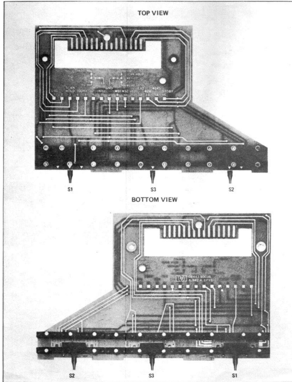
Figure 8-44. A16, Switch Assembly (8443A)
