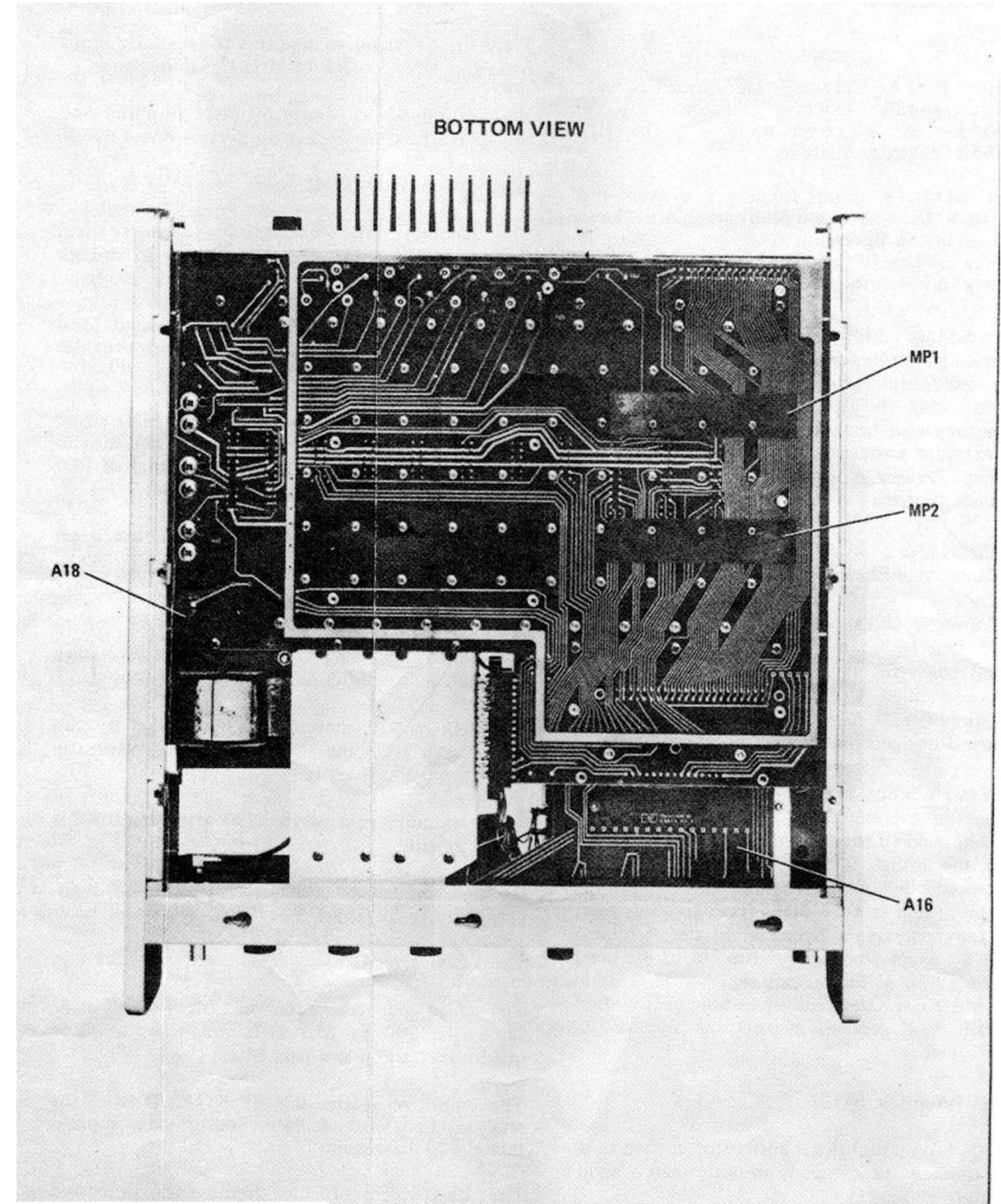
Figure 8-18. Chassis Mounted Parts and Assembly Locations
