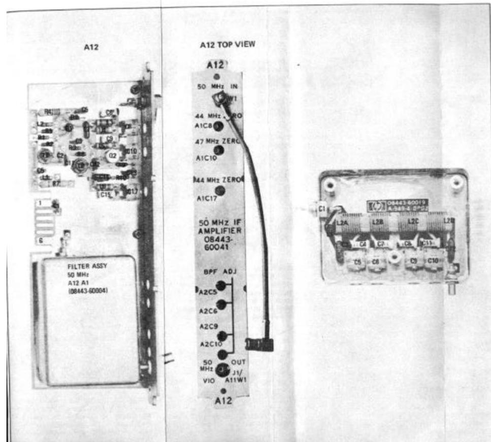
Figure 8-22. A12, 50 MHz Amplifier, Cover and Components
