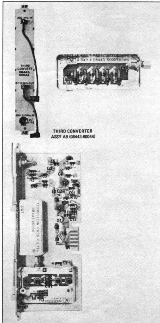
Figure 8-25. A9, Third Converter Assembly
