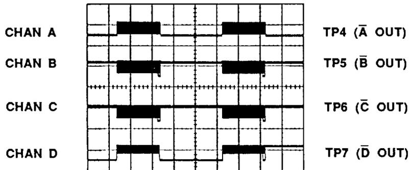
Figure SS84. Output Waveforms, MARKER Mode (CHANGE 10)
