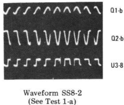
each channel and the TIME/DIV to 1 μSec, Trigger INT, ACF and SLOPE +. The waveform should be as shown in waveform SS8-2. If none of the waveforms are present, check the switching matrix. If waveform A is present and B and C are not, check Q1 and associated components. If waveform A and B are present and C is not, check Q2 and associated components. If all of the waveforms are present, proceed to test procedure .
