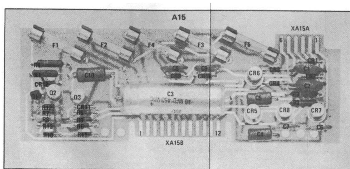
Figure 8-29. A15, Rectifier Assembly, Components
