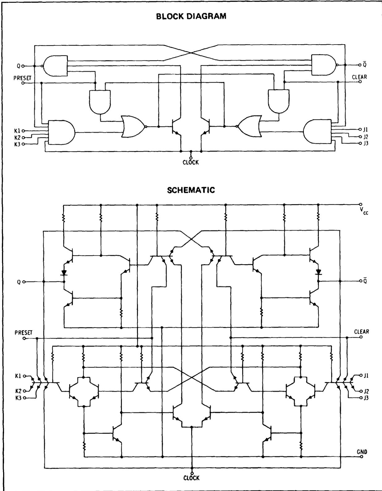
Figure 8-10. JK Master-Slave flip-flop (Typical)
