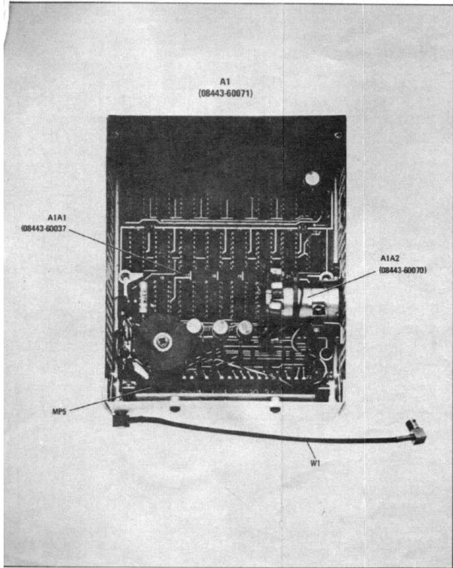
Figure 8-40. A1, Low Frequency Counter Assembly, Components
