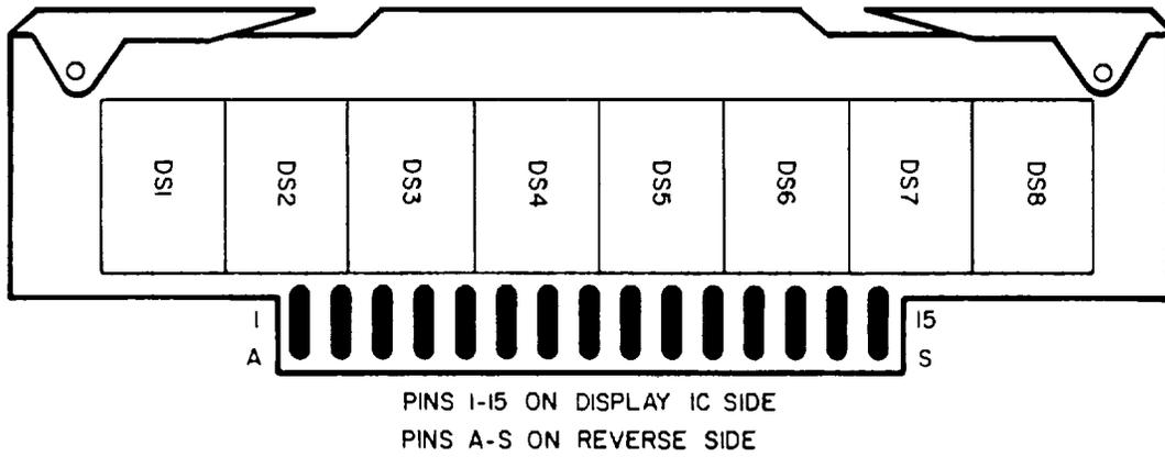
Figure 8-38B. A1A2, Counter Display Board Assembly, Components (CHANGE 9)
