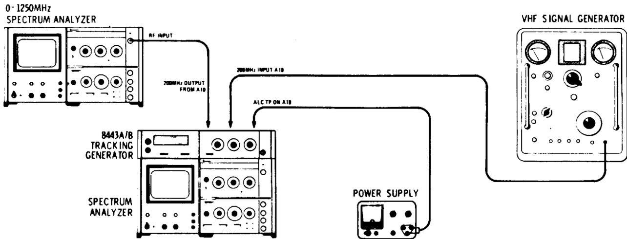
Figure 5-3. 200 MHz IF Test Setup
