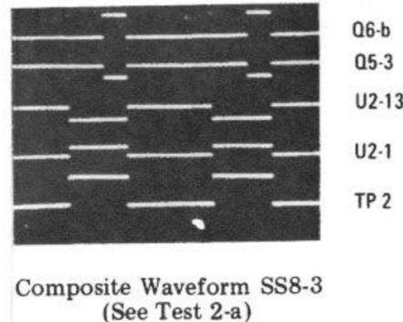
set to 100 Hz. Set the analyzer SCAN TIME PER DIVISION to 1 MILLISECOND. Synchronize the oscilloscope to the analyzer scan, triggered on + slope, ACF. Waveform SS8-3 is a composite waveform for the five critical circuit points; these points are identified directly below the composite waveform. Oscilloscope VOLTS/DIV information follows identification of test points.
