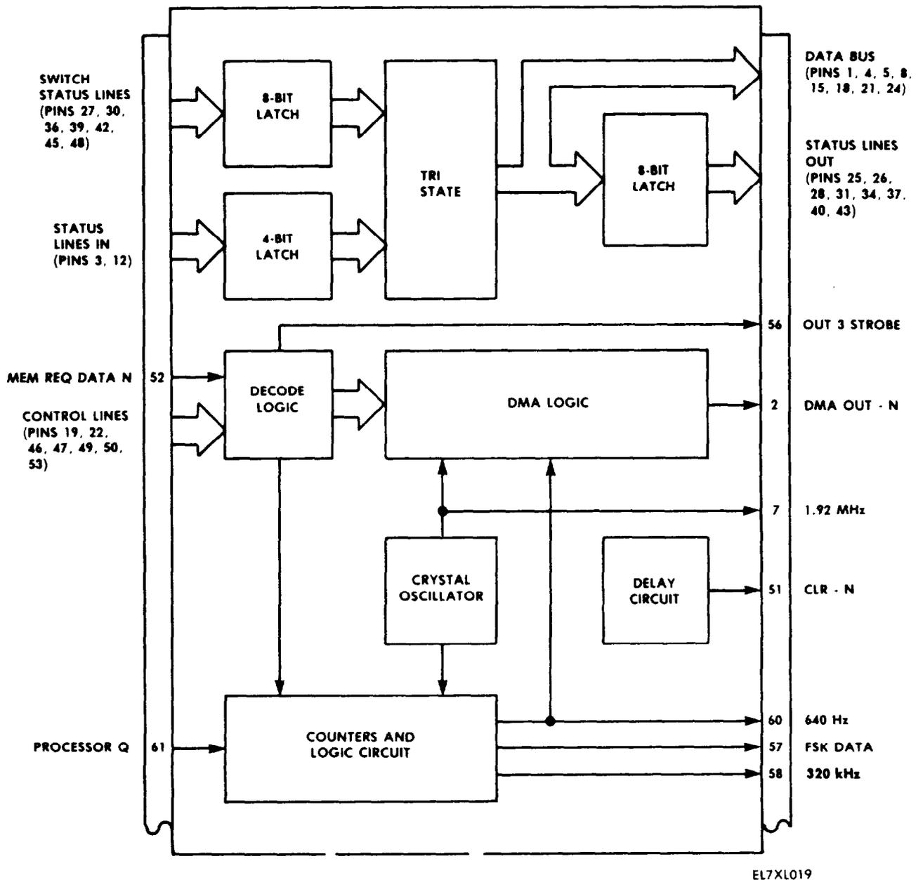
Figure 5-3. Decoder/Timer Functional Block Diagram.
