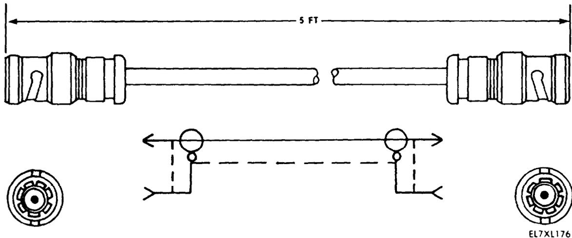
Figure 9-5. Test Cables (Sheet 6 of 6)
