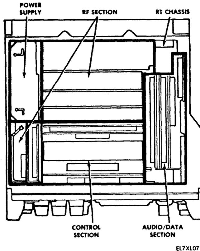
Figure 2-2. RT Partitioning of Functional Sections
