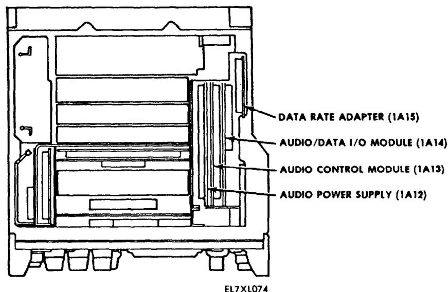
Figure 2-5. Audio/Data Section Module locations
