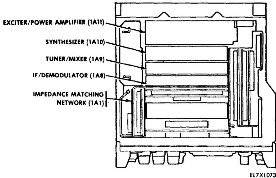
Figure 2-4. RF Section Module Locations
