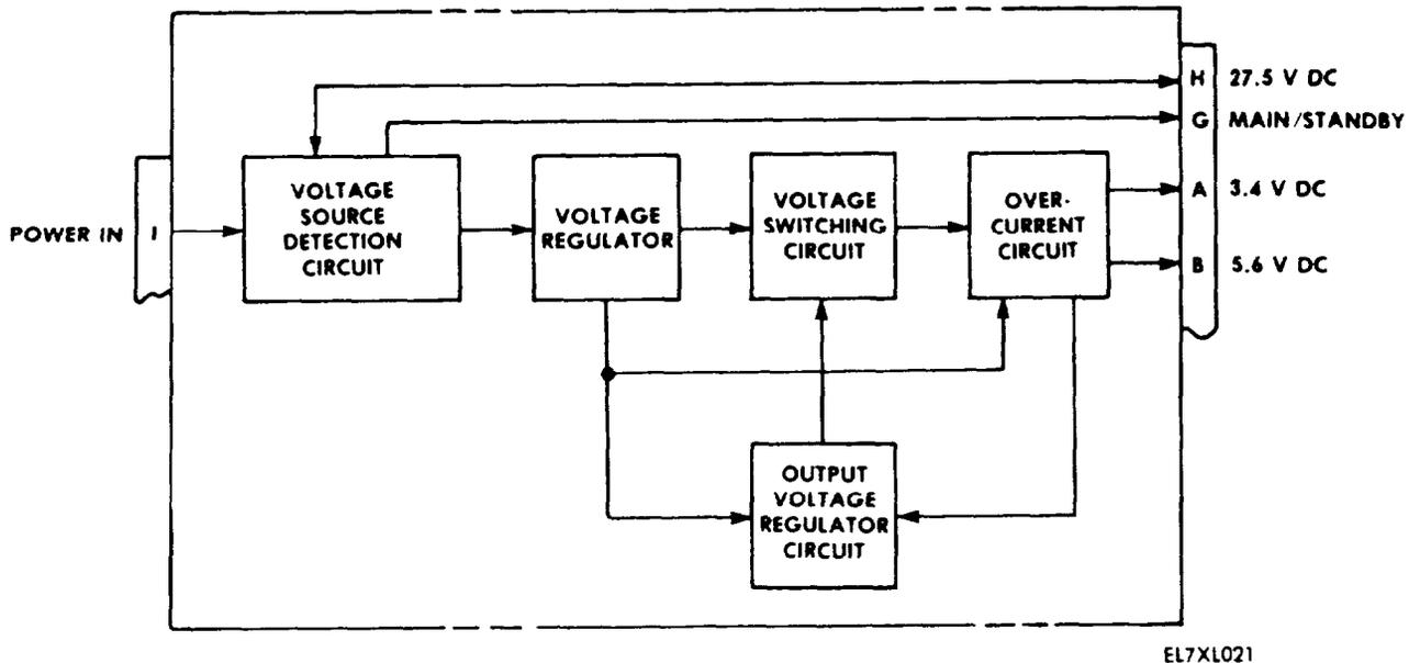
Figure 5-5. Power Supply Functional Block Diagram.
