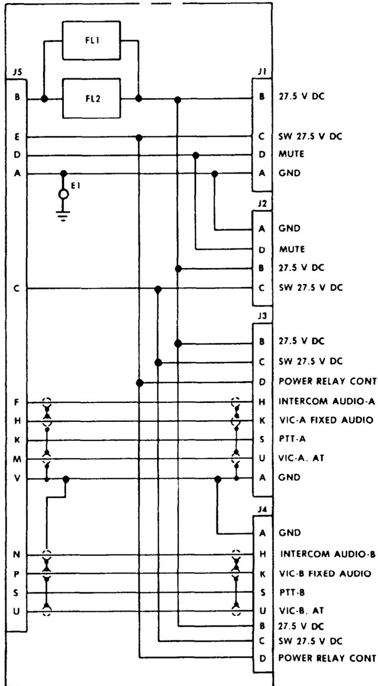
Figure 6-1. Electrical Connector Assembly Schematic Diagram.
