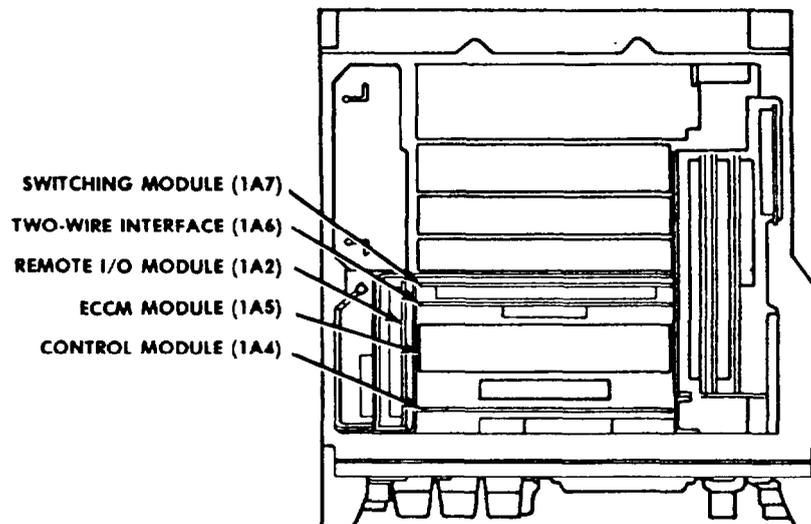
Figure 2-3. Control Section Module Locations
