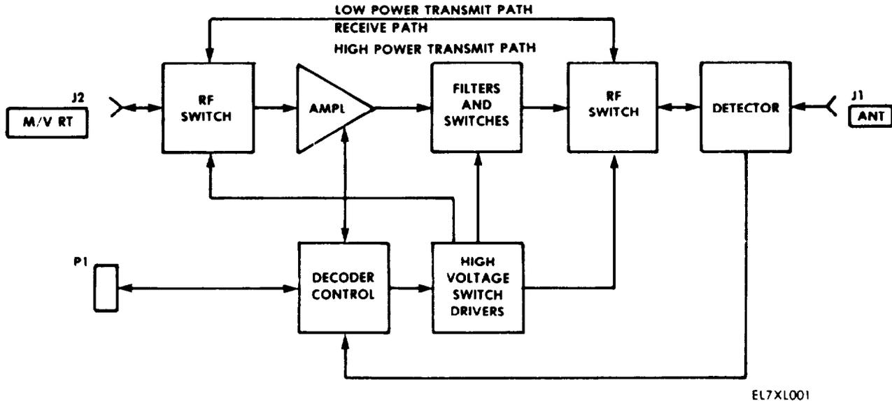
Figure 4-1. Power Amplifier Block Diagram.
