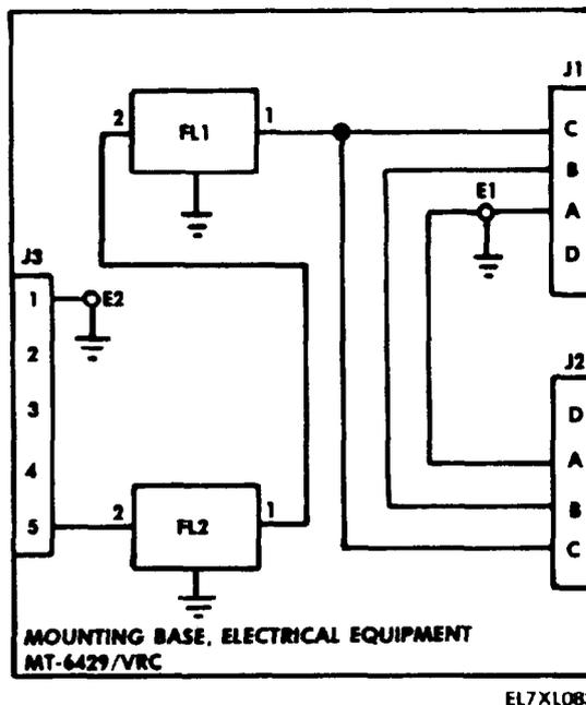
Figure 10-1. COMSEC Mount Schematic Diagram.
