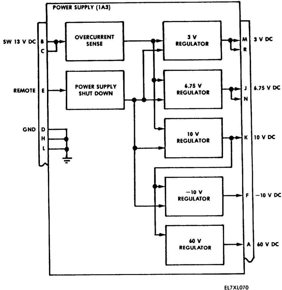
Figure 2-7. Power Supply Functional Block Diagram
