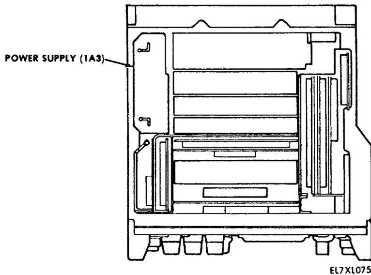
Figure 2-6. Power Supply Location
