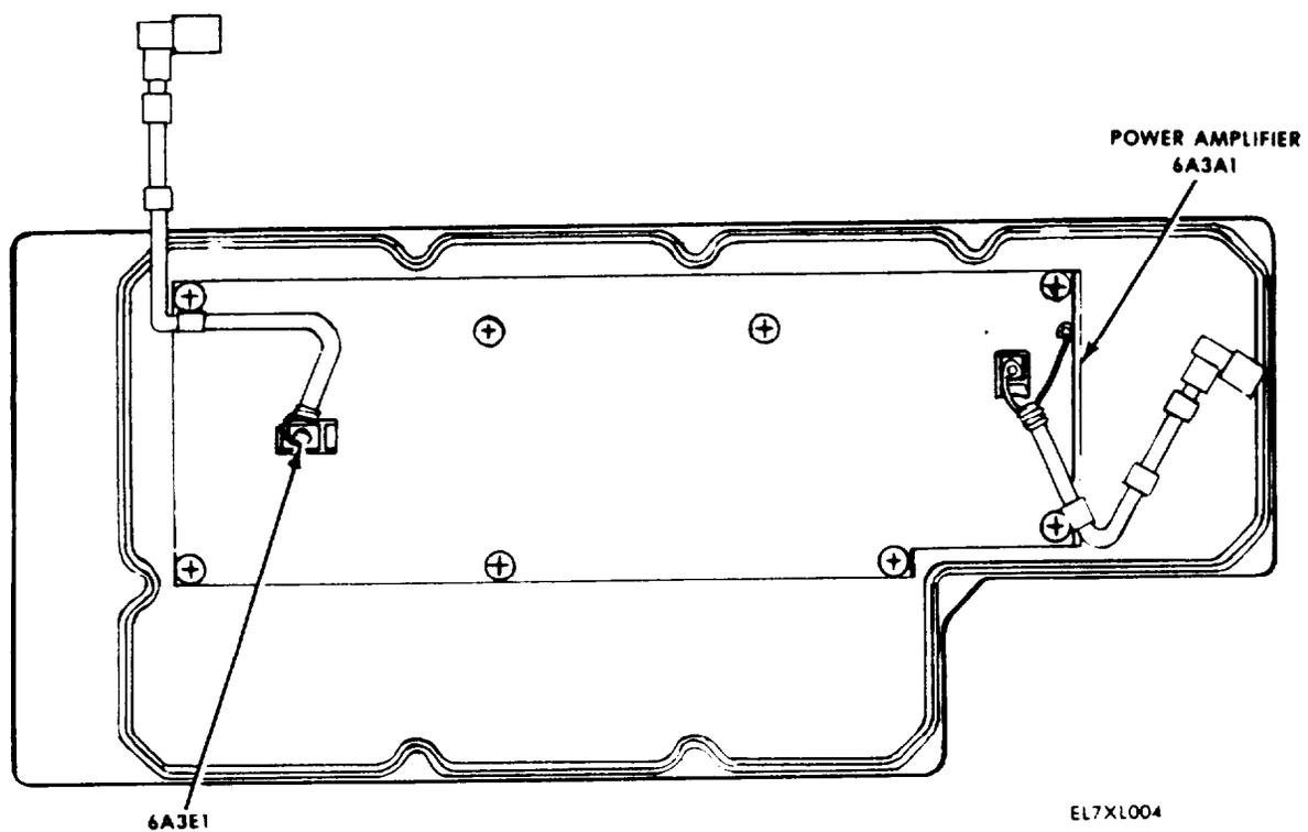
Figure 4-4. Test Point Locations for Power Amplifier Heat Sink (6A3)
