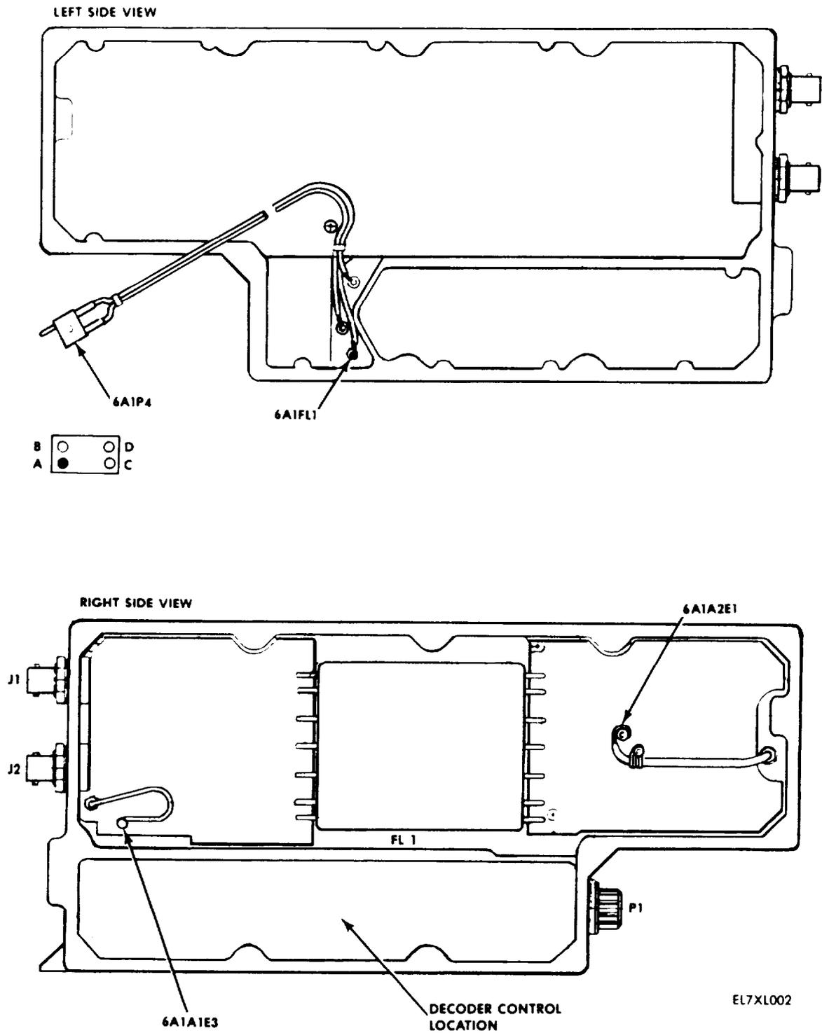
Figure 4-3. Test Point Locations in Power Amplifier Case (6A1)
