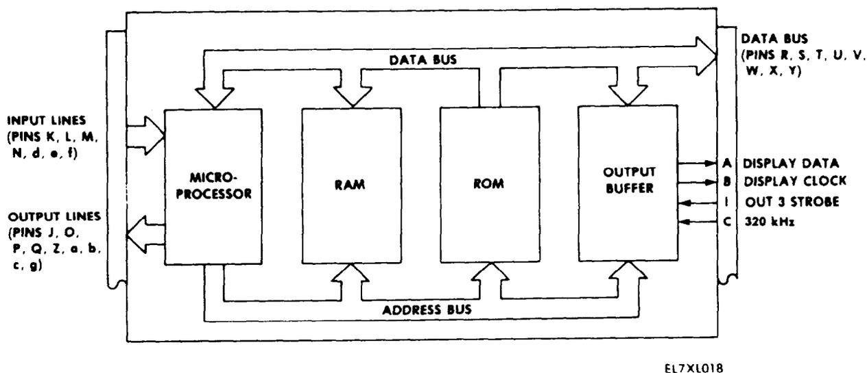
Figure 5-2. Microcontroller Functional Block Diagram.
