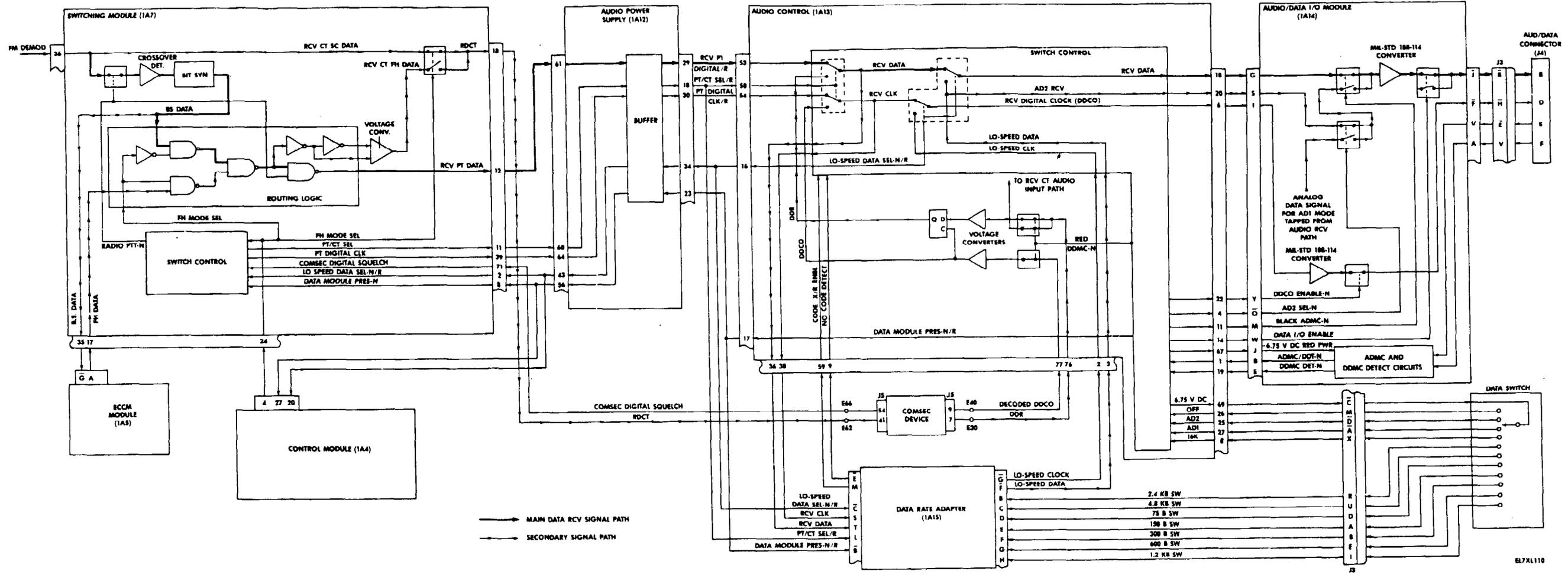
FO-5. RT Data Receive Signal Path Functional Block Diagram
