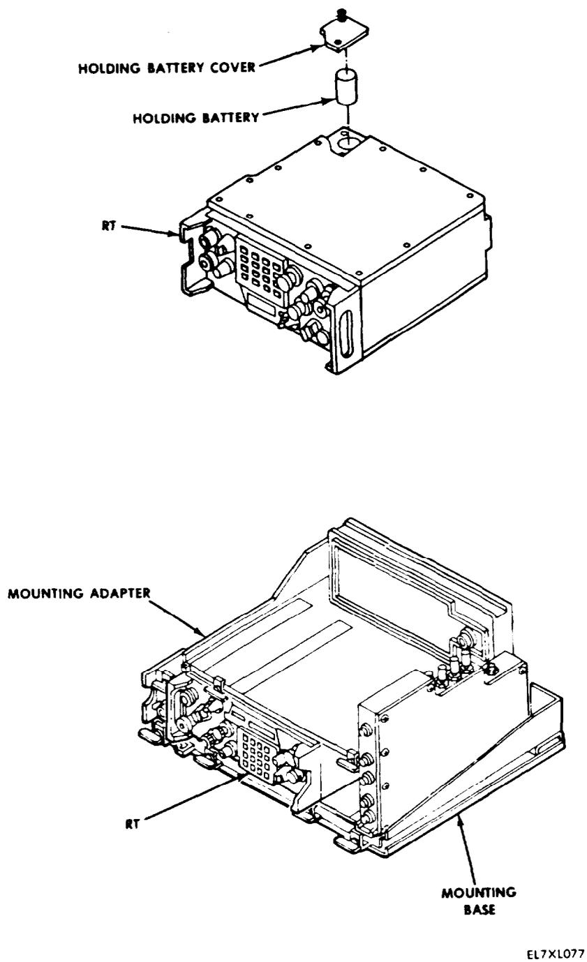
Figure 9-3. Assembly and Installation of Test Radio (Sheet 2 of 2)
