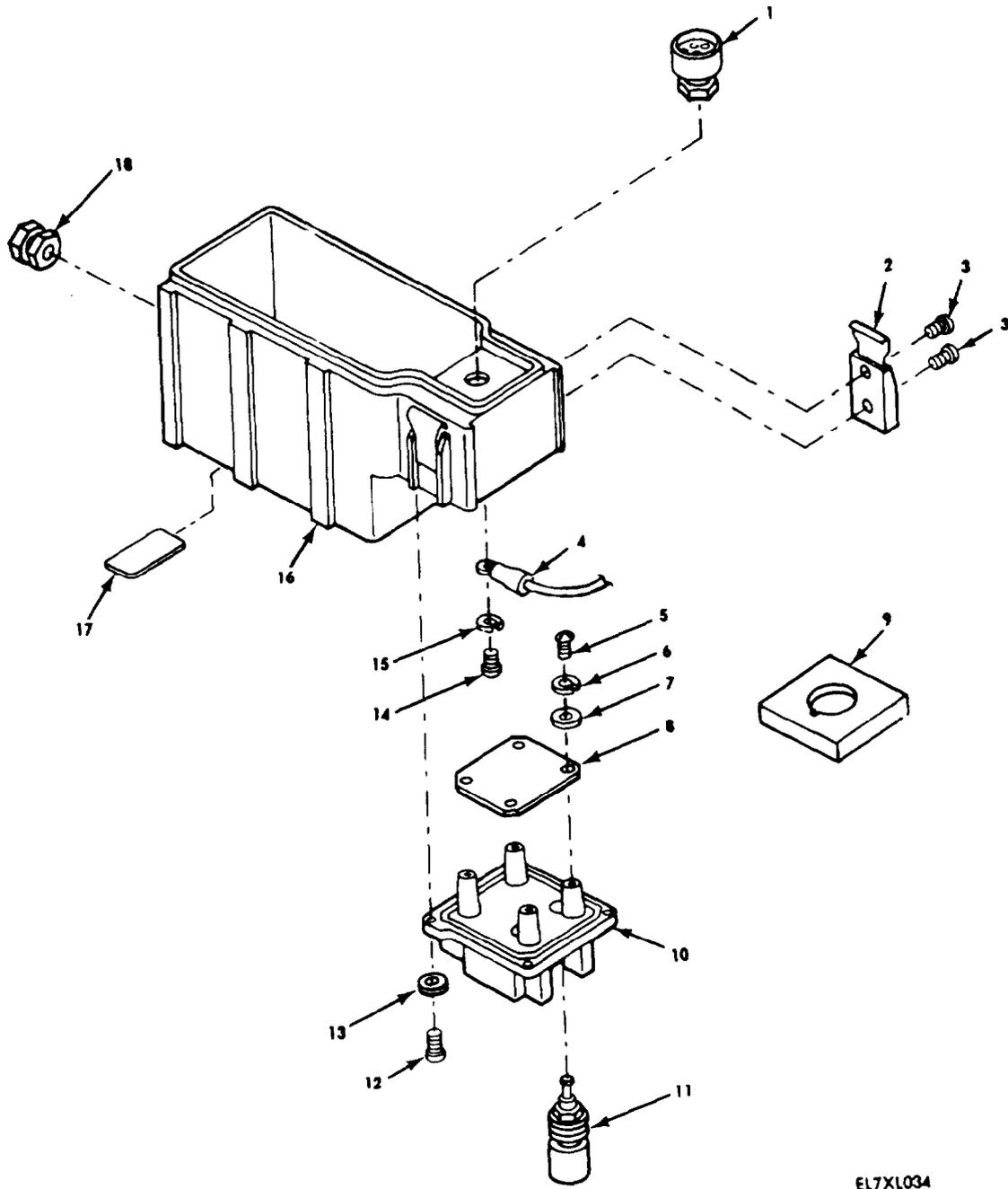
Figure 7-3. Battery Box CY-8346/PRC
