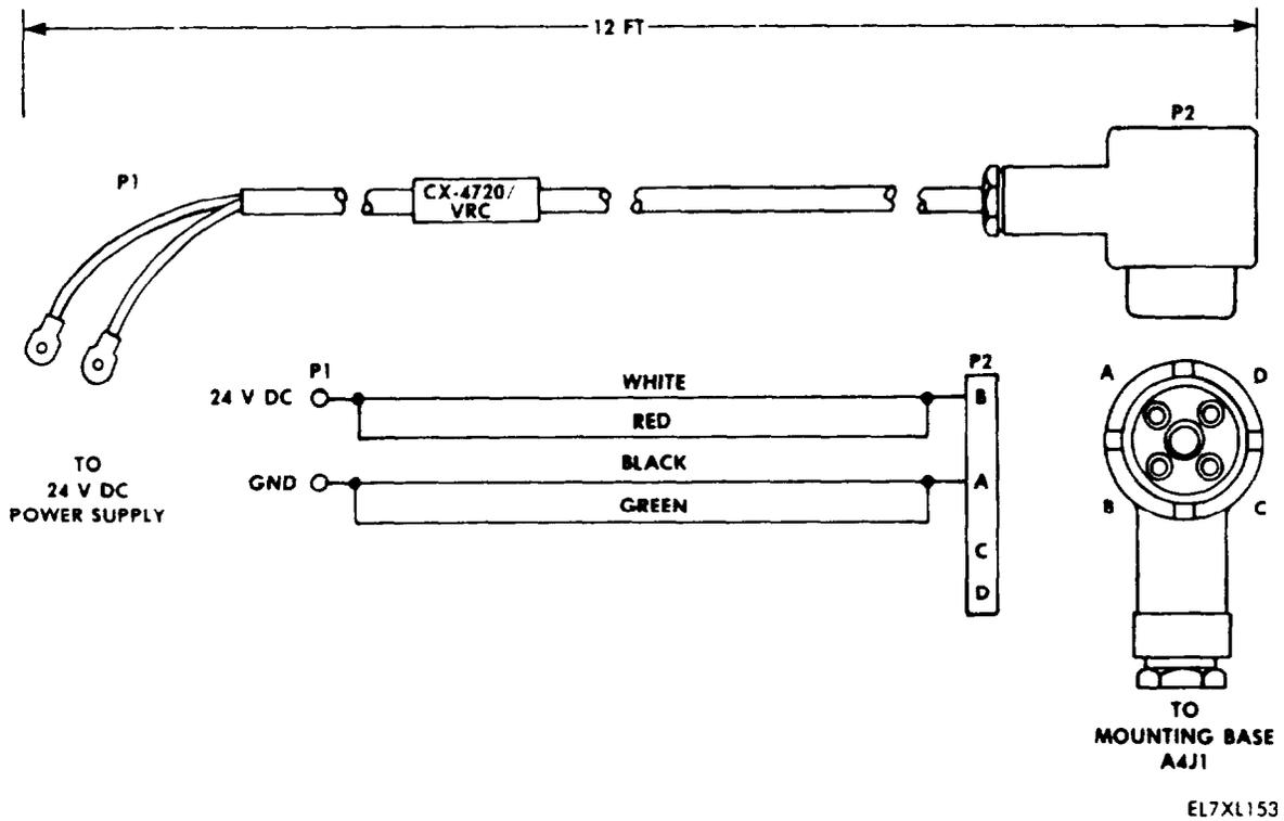
Figure 9-2. Test Cables (Sheet 5 of 6)
